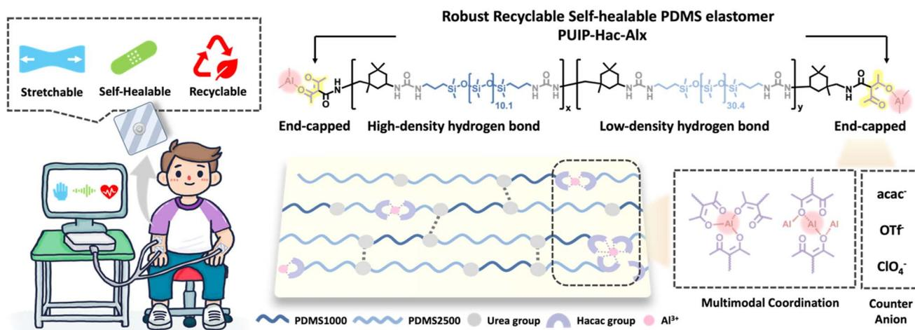
Fig. 1 Designed structure and schematic illustrating the dynamic intermolecular interaction and properties of PUIP-Hac, PUIP-Hac-Alac, ALOTf and AlClO<sub>4</sub> polymers.
