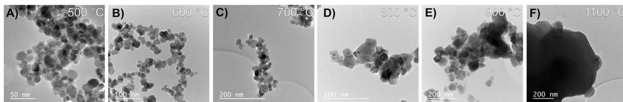
Fig. 4 TEM micrographs representative of the morphology of the  $\text{Ni}_{0.6}\text{Zn}_{0.4}\text{Fe}_2\text{O}_4$  particles obtained after calcination at (A) 500 °C, (B) 600 °C, (C) 700 °C, (D) 800 °C, (E) 900 °C and (F) 1100 °C.
