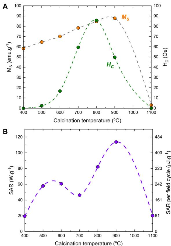
Fig. 5 (A) Magnetic properties and (B) SAR generated by the  $\text{Ni}_{0.6}\text{Zn}_{0.4}\text{Fe}_2\text{O}_4$  ferrites nanoparticles obtained by calcination of the hydroxide precursor at different temperatures.
