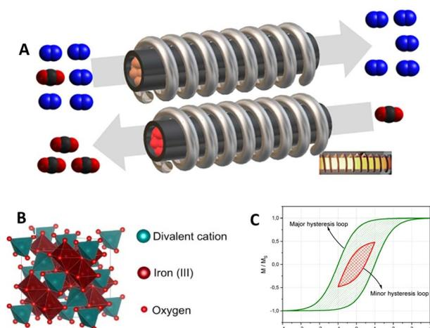
Fig. 1 (A) Schematic of IHSA setup operating a CO<sub>2</sub>/N<sub>2</sub> separation process, (B) structure of a spinel ferrite unit cell, and (C) magnetisation curves displaying major and minor hysteresis loops.
