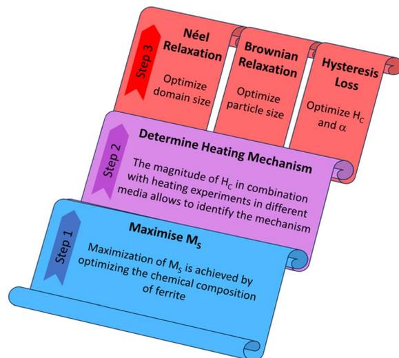
Fig. 2 Optimization of the heating efficiency of ferrite materials can be achieved through (step 1) the maximization of their saturation magnetization ( $M_S$ ), (step 2) the determination of the involved heating mechanism and (step 3) a mechanism-dependent optimization of their morphological and magnetic properties.
