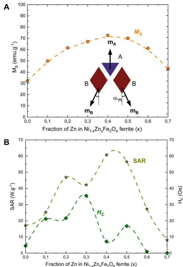
**Fig. 3** Evolution of the magnetic properties and hysteresis heat generated by Ni<sub>1-x</sub>Zn<sub>x</sub>Fe<sub>2</sub>O<sub>4</sub> ferrites with varying Zn(II) substitution grades ( $x$ ). (A) Saturation magnetization. The inset illustrates the Yafet-Kittel rearrangement leading to an increase in the canting angle  $\alpha_{YK}$  and a reduction in  $M_S$  and in the SAR when  $x > 0.4$ . (B) SAR generated by the ferrites and their coercivity.
