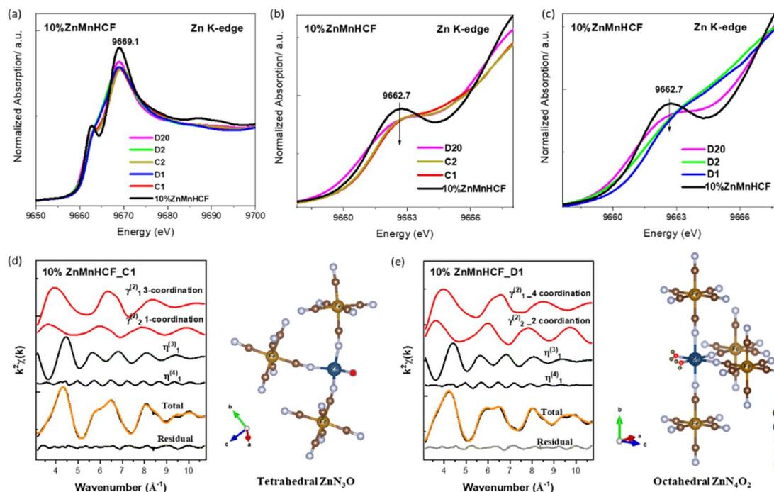
**Fig. 6** *Ex situ* XANES of (a) the Zn K-edge and (b and c) zoom-in of the Zn K-edge XANES. EXAFS fitting results at Zn K-edge for (d) 10% ZnMnHCF\_C1 based on a tetrahedral coordination of Zn sites, with 3 N from -NC- ligands and 1 O from H<sub>2</sub>O and (e) 10% ZnMnHCF\_C2 electrodes, based on an octahedral coordination of Zn sites, with 4 N from -NC- ligands and 2 O from H<sub>2</sub>O.
