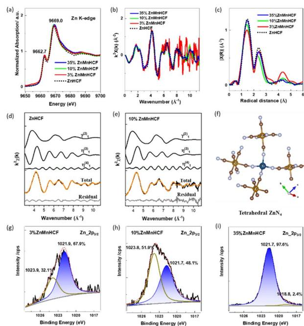
Fig. 3 (a) XANES spectra of Zn K-edge of Zn-substituted MnHCF samples and pure ZnHCF sample. (b)  $k^2$ -Weighted EXAFS signals, as well as (c) corresponding Fourier transform (FT) of  $k^2$ -weighted EXAFS signal of Zn K-edge. EXAFS analysis of Zn K-edge of (d) ZnHCF and (e) 10% ZnMnHCF samples. (f) The tetrahedral coordination of Zn sites. Zn  $2p_{3/2}$  XPS data of (g) 3% ZnMnHCF, (h) 10% ZnMnHCF and (i) 35% ZnMnHCF samples.
