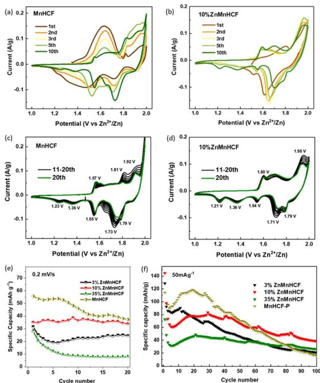
Fig. 4 CV data of (a and c) MnHCF and (b and d) 10% ZnMnHCF in the 3 M ZnSO<sub>4</sub> electrolyte at 0.2 mV s<sup>−1</sup> for 20 cycles. (e) The specific capability calculated based on CV data. (f) Cycling stability of Zn-substituted MnHCF samples at 50 mA g<sup>−1</sup>.
