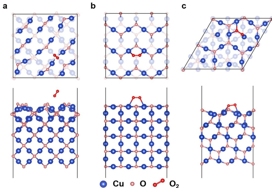
Fig. 6 The most stable  $\text{O}_2$  adsorption configurations on  $\text{Cu}_2\text{O}$  (a)  $\{100\}$ , (b)  $\{110\}$ , and (c)  $\{111\}$  surfaces. The upper and lower panels show the top and side views, respectively.
