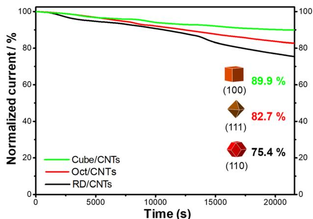
Fig. 5 Chronoamperometric curves for the Cu<sub>2</sub>O/CNTs catalysts measured at 0.65 V vs. RHE in an O<sub>2</sub>-saturated 0.1 M KOH solution.
