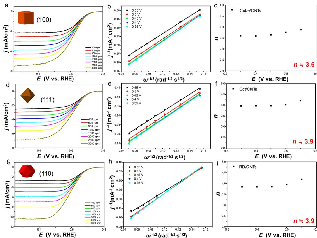
Fig. 4 LSV polarization curves for the ORR at different rotation speeds, the corresponding Koutecký–Levich plots ( $j^{-1}$  vs.  $\omega^{-1/2}$ ) at different potentials, and plots of the transferred electron numbers versus potentials for (a–c) Cu<sub>2</sub>O cubes, (d–f) octahedra and (g–i) rhombic dodecahedra mixed with CNTs.
