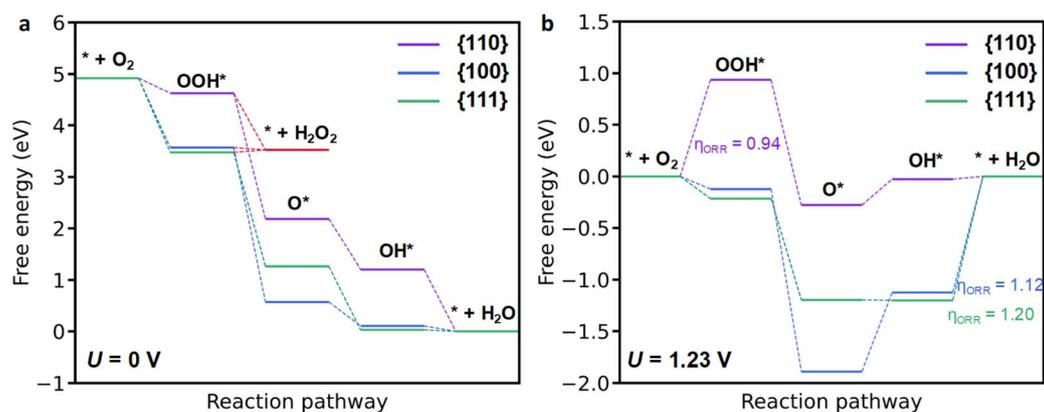
Fig. 7 Free energy diagram for oxygen reduction on  $\text{Cu}_2\text{O}$   $\{100\}$ ,  $\{110\}$ , and  $\{111\}$  surfaces with (a)  $U = 0$  V and (b)  $U = 1.23$  V. The theoretical overpotential ( $\eta_{\text{ORR}}$ ) and the corresponding potential-determining step are presented in panel (b).
