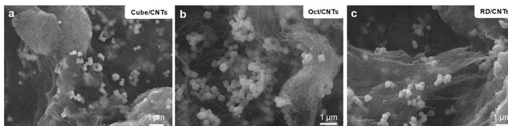
Fig. 1 SEM images of Cu<sub>2</sub>O (a) cubes, (b) octahedra, and (c) rhombic dodecahedra mixed with carbon nanotubes.
