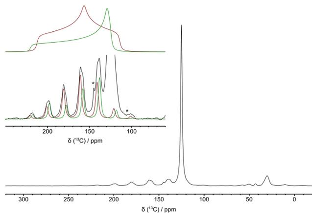
Fig. 5  $^{13}\text{C}$  DE MAS spectrum of amine-PIM-1 loaded with  $^{13}\text{CO}_2$  recorded using a MAS frequency of 2.5 kHz. In the inset, simulations of the side band manifolds of signals of carbamic acids with  $\delta_{\text{iso}}$  of 158 and 161 ppm (bottom) and the corresponding reconstructed chemical shift tensors (top) are shown in green and red, respectively. Asterisks indicate spinning side bands of physisorbed  $\text{CO}_2$  undergoing anisotropic motion.
