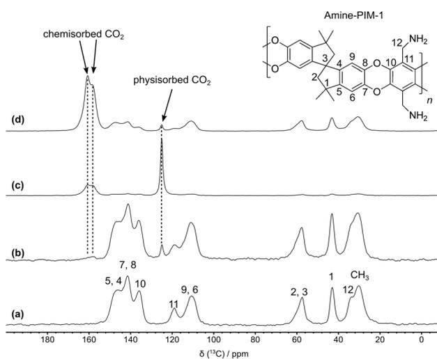
Fig. 2 Quantitative <sup>13</sup>C DE MAS spectra of: (a) amine-PIM-1; (b) amine-PIM-1 loaded with CO<sub>2</sub>; (c) amine-PIM-1 loaded with <sup>13</sup>CO<sub>2</sub>. (d) <sup>1</sup>H-<sup>13</sup>C CP MAS spectrum of amine-PIM-1 loaded with <sup>13</sup>CO<sub>2</sub> recorded with a contact time of 2 ms. All the spectra were acquired at 298 K at a spinning frequency of 15 kHz.
