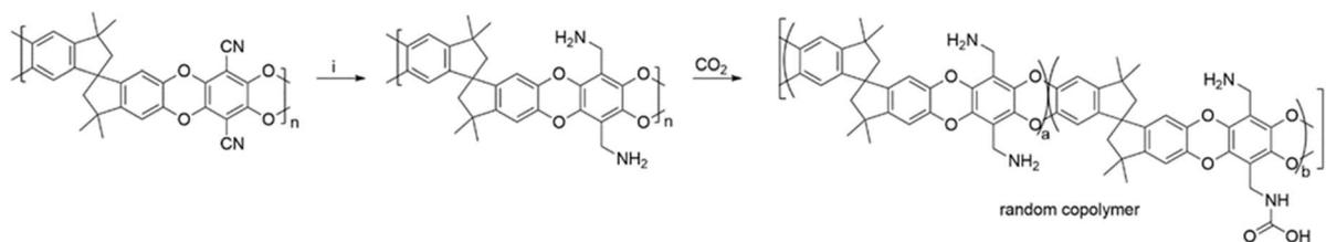
Scheme 1 Post-modification of PIM-1 to give amine-PIM-1 and formation of chemisorbed-amine-PIM-1 following CO<sub>2</sub> loading. (i) borane dimethyl sulphide 5.0 M in diethyl ether.
