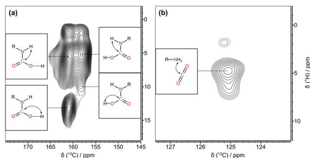
Fig. 4 Expansion of the <sup>1</sup>H-<sup>13</sup>C HETCOR MAS spectra of chemisorbed-amine-PIM-1 loaded with <sup>13</sup>CO<sub>2</sub> recorded with a contact time of (a) 0.5 ms and (b) 1.5 ms.
