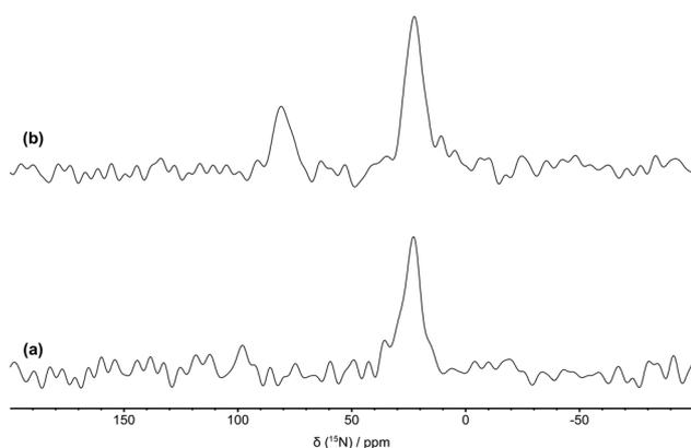
Fig. 3 <sup>1</sup>H-<sup>15</sup>N CP MAS spectra recorded with a contact time of 4 ms on: (a) pristine amine-PIM-1 membrane and (b) amine-PIM-1 membrane loaded with CO<sub>2</sub> (i.e., chemisorbed-amine-PIM-1). The spectra were acquired at 298 K at a spinning frequency of 8 kHz.
