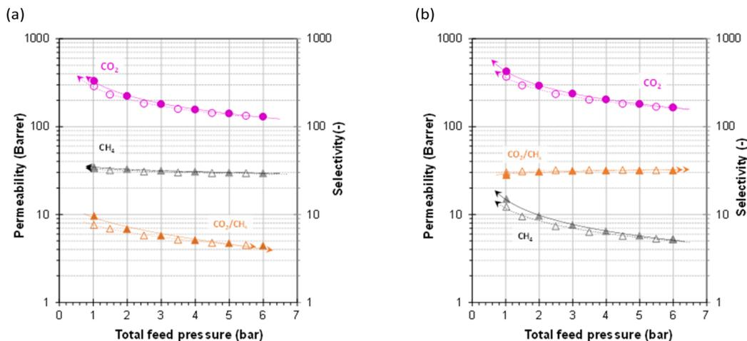
Fig. 1 Pressure dependence of permeability and selectivity in amine-PIM-1 for (a) pure CO<sub>2</sub> and CH<sub>4</sub>, and (b) for a CO<sub>2</sub>/CH<sub>4</sub> mixture (52.11/47.89 vol%). Filled symbols represent the pressure-increase steps and open symbols represent the subsequent pressure-decrease steps.
