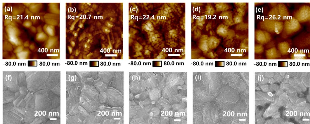
Fig. 4 Surface morphology characterization of perovskite films. (a–e) AFM images of (a) control film, (b) PEAI-treated film, (c) *o*-FPEAI-treated film, (d) *m*-FPEAI-treated film, and (e) *p*-FPEAI-treated film. (f–j) Top-view SEM images of (f) control film, (g) PEAI-treated film, (h) *o*-FPEAI-treated film, (i) *m*-FPEAI-treated film, and (j) *p*-FPEAI-treated film.
