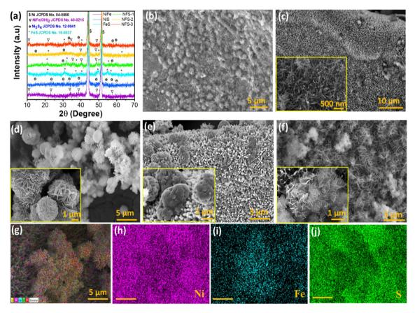
Fig. 1 (a) XRD pattern of the  $Ni_x$ Fe<sub>1-x</sub>-hydroxide/sulphide heterostructure, (b-g) FE-SEM images of (b) NiS@NF, (c) FeS@NF, (d)  $NiFe(OH)_2@NF$ , (e) NFS-1@NF, and (f) NFS-2@NF, and (q-j) EDS elemental mapping images of NFS-2@NF catalysts.
