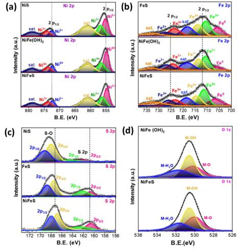
Fig. 2 XPS spectra of the Ni<sub>x</sub>Fe<sub>1-x</sub>-hydroxide/sulphide heterostructure: (a) Ni 2p, (b) Fe 2p, (c) S 2p, and (d) O 1s.
