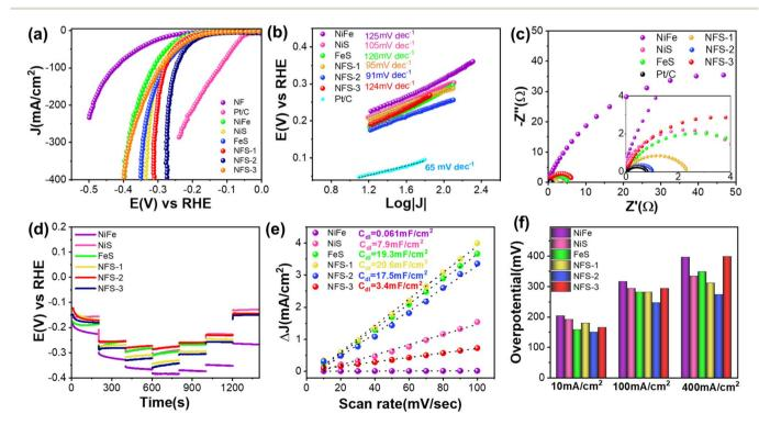
Fig. 3 HER performance of Ni<sub>x</sub>Fe<sub>1-x</sub>-hydroxide/sulphide in 1.0 M KOH: (a) LSV polarization curves of Ni<sub>x</sub>Fe<sub>1-x</sub>-hydroxide/sulphide, NF and Pt/C. (b) Tafel plots, (c) EIS graph, (d) accelerated chrono at 10, 100, 200 and 300 mA cm<sup>-2</sup>, (e)  $C_{\rm cl}$  graph, (f) overpotential table at 10, 100 and 400 mA cm<sup>-2</sup>.
