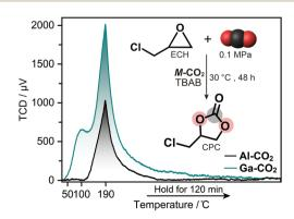
Fig. 3 NH<sub>3</sub>-TPD profiles of M-CO<sub>2</sub>. Inset: conversion of ECH into CPC via CO<sub>2</sub> cycloaddition reaction using M-CO<sub>2</sub> catalysis with TBAB as a co-catalyst.
