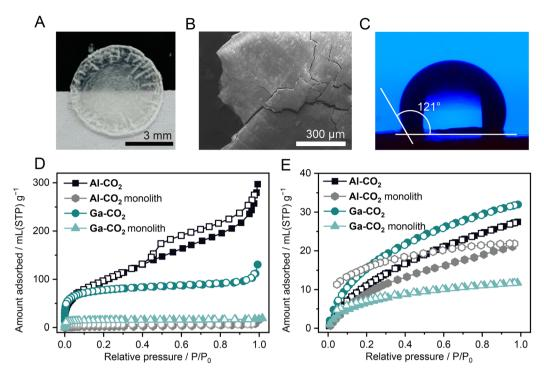
Fig. 4 (A) Optical image of the transparent Al-CO<sub>2</sub> monolith with a diameter of 7.0 mm. (B) SEM image of the Al-CO<sub>2</sub> monolith. (C) Image of a water droplet on the surface of the Al-CO<sub>2</sub> monolith. (D) N<sub>2</sub> and (E) H<sub>2</sub> adsorption isotherms at 77 K for M-CO<sub>2</sub> powder and monoliths. Solid/open symbols indicate adsorption/desorption isotherms, respectively.
