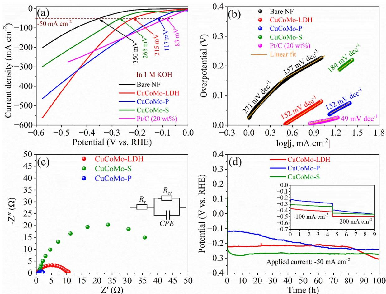
Fig. 5 HER studies: (a) LSV curves at a 2 mV s<sup>-1</sup> scan rate, (b) Tafel plots, (c) Nyquist plots, and (d) chronopotentiometric stability test profiles.
