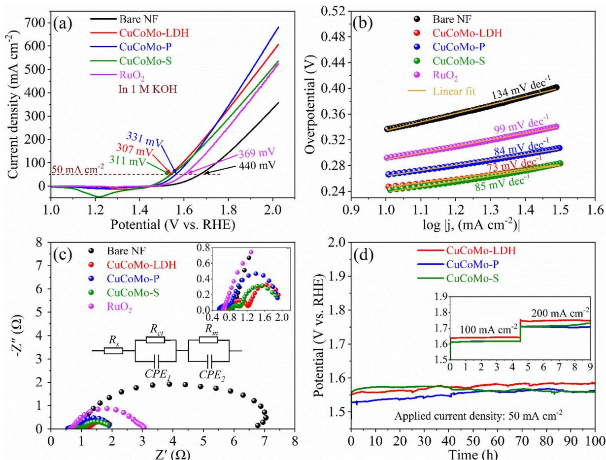
Fig. 4 OER studies: (a) LSV curves at a 2 mV s<sup>-1</sup> scan rate, (b) Tafel plots, (c) Nyquist plots, and (d) chronopotentiometric stability test profiles.
