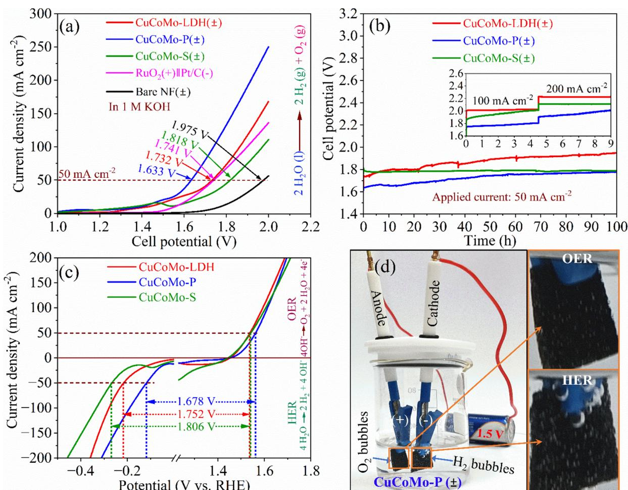
Fig. 7 OWS studies: (a) LSV curves of the fabricated electrolyzers at a  $2 \text{ mV s}^{-1}$  scan rate, (b) chronopotentiometric stability test of the fabricated electrolyzers, (c) half-cell HER and OER LSV curves plotted together, and (d) OWS performed with the CuCoMo-P(±) electrolyzer powered by a 1.5 V AA battery.
