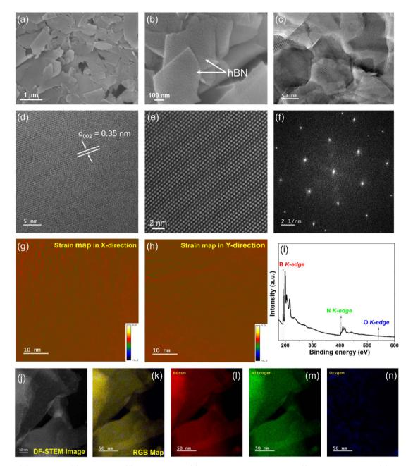
Fig. 2 (a and b) SEM images, (c) TEM image, (d) HRTEM image, (e) atomic-scale HRTEM image, (f) corresponding FFT, (g) strain map in Xdirection, (h) strain map in Y-direction, (i) core-loss EELS spectra, (j) STEM-HADDF image, and (k-n) EELS elemental mapping of the HPHprepared 2D hBN flakes.
