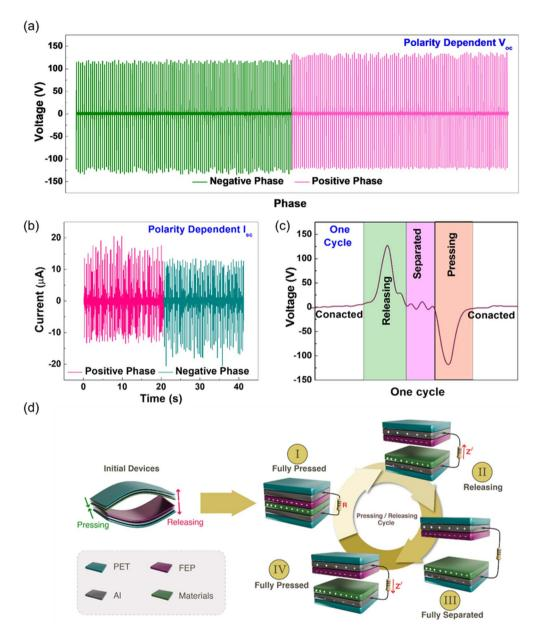
Fig. 4 Polarity dependent (a) open circuit voltage, (b) short circuit current, (c) one complete cycle showing the smooth output signal, and (d) mechanism of output characteristics.
