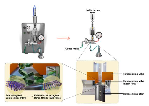
Schematic illustration of the HPH process for preparing scalable 2D hBN flakes
