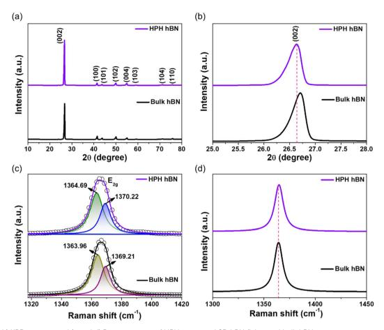
Fig. f 1 (a and b) XRD patterns and (c and d) Raman spectra of HPH processed 2D hBN flakes and bulk hBN.
