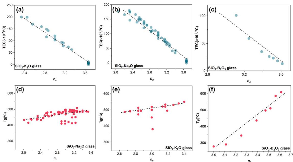
Fig. 2 Thermal expansion coefficients of SiO<sub>2</sub>-K<sub>2</sub>O (a), SiO<sub>2</sub>-Na<sub>2</sub>O (b), and SiO<sub>2</sub>-B<sub>2</sub>O<sub>3</sub> (c) glass and glass transition temperatures of SiO<sub>2</sub>-K<sub>2</sub>O (d), SiO<sub>2</sub>-Na<sub>2</sub>O (e), and SiO<sub>2</sub>-B<sub>2</sub>O<sub>3</sub> (f) as a function of the topology constraint parameter  $n_c$ .
