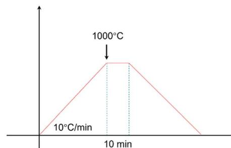
Fig. 8 Thermal schedule for the sealing-melting process.
