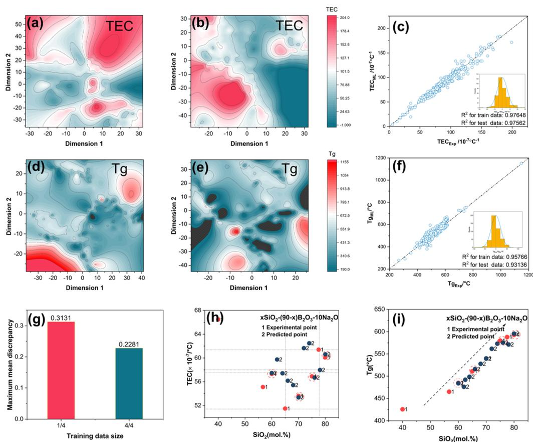
Fig. 3 *t*-SNE analysis of the training data with (a and d) and without (b and e) topology-informed descriptors; performance of ML models on (c) TEC and (f)  $T_g$  predictions. Insets represent distribution of error between the predicted and experimental values; (g) effects of training size on the maximum mean discrepancy between the domain and target; the experimental and predicted (h) TEC and (i)  $T_g$  values of  $x\text{SiO}_2-(90-x)\text{B}_2\text{O}_3-10\text{Na}_2\text{O}$  system.
