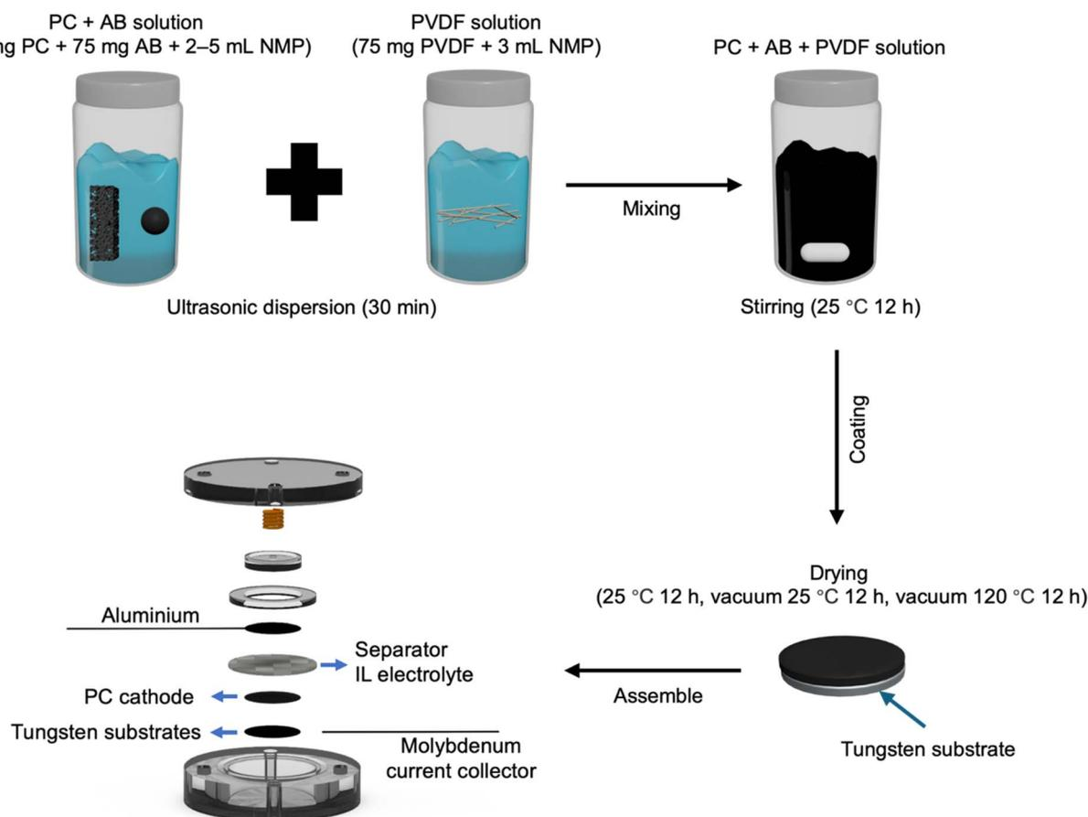
Fig. 2 Preparation of cathodes and assembly of porous carbon/aluminium polytetrafluoroethylene cell. PC, porous carbon; AB, acetylene black; PVDF, polyvinylidene fluoride; NMP, of *N*-methyl-2-pyrrolidone; IL, ionic liquid.
