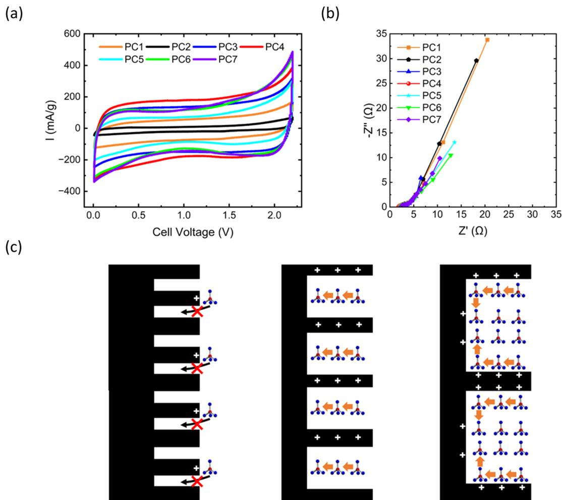
Fig. 4 Rechargeable porous carbon/aluminium cell. (a) Cyclic voltammetry of Al foil and PC at a scan rate of 1 mV s<sup>-1</sup>. (b) Nyquist plots of PC1–7 at 2.2 V and at an amplitude of 10.0 mV and frequencies ranging from 1.0 MHz to 0.1 Hz. (c) Model diagram of the adsorption of AlCl<sub>4</sub><sup>-</sup> ions on the PC cathodes. PC1 (YP50F), PC2 (MSP-20), PC3 (MSA-20), PC4 (MSC-30), PC5 (CNovel 20 nm), PC6 (CNovel MJ4 010-00), and PC7 (CNovel MH-00); PC, porous carbon.
