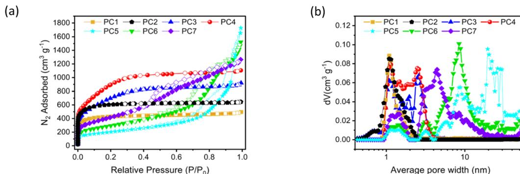
**Fig. 1** Nitrogen adsorption–desorption isotherms (a) and pore size distribution curves (b) for porous carbon materials PC1, PC2, PC3, PC4, PC6, and PC7. PC1 (YP50F), PC2 (MSP-20), PC3 (MSA-20), PC4 (MSC-30), PC5 (CNovel 20 nm), PC6 (CNovel MJ4 010-00), and PC7 (CNovel MH-00).
