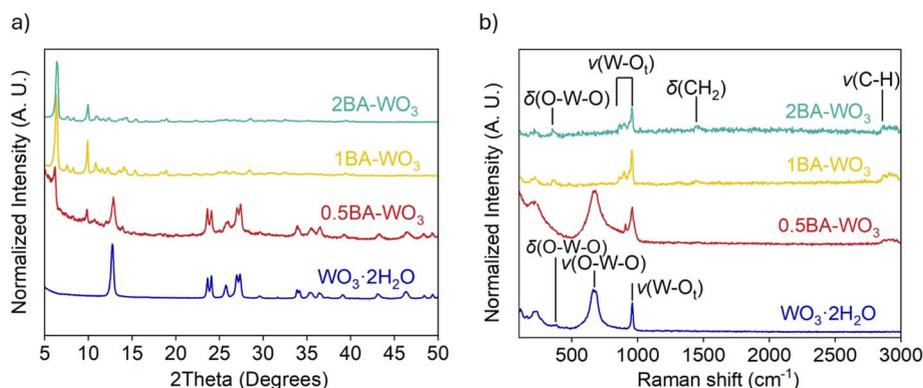
Fig. 1 (a) XRD and (b) Raman spectroscopy of  $\text{WO}_3 \cdot 2\text{H}_2\text{O}$  and BA-pillared  $\text{WO}_3$  obtained from syntheses using different ratios of butylamine to  $\text{WO}_3 \cdot 2\text{H}_2\text{O}$ .
