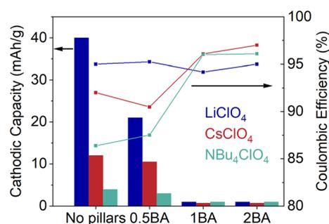
Fig. 8 Cathodic capacity and coulombic efficiency of  $\text{WO}_3 \cdot n\text{H}_2\text{O}$ , pillared tungsten oxides  $0.5\text{BA-WO}_3$ ,  $1\text{BA-WO}_3$  and  $2\text{BA-WO}_3$  in different non-aqueous electrolytes.
