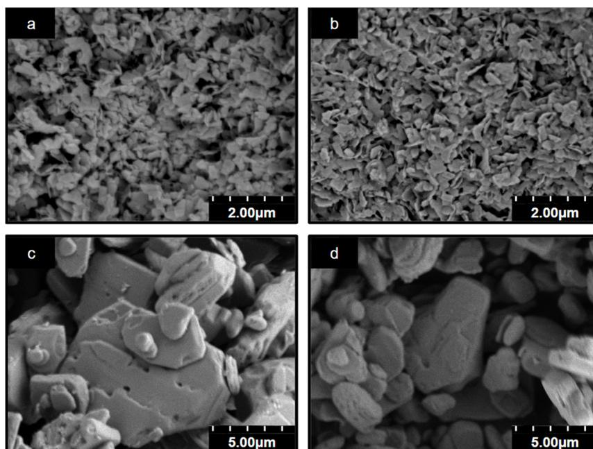
Fig. 2 SEM of the precursor  $\text{WO}_3 \cdot 2\text{H}_2\text{O}$  (a) and BA-pillared tungsten oxides obtained from syntheses with various ratios of butylamine: (b) 0.5BA- $\text{WO}_3$ , (c) 1BA- $\text{WO}_3$ , and (d) 2BA- $\text{WO}_3$ .
