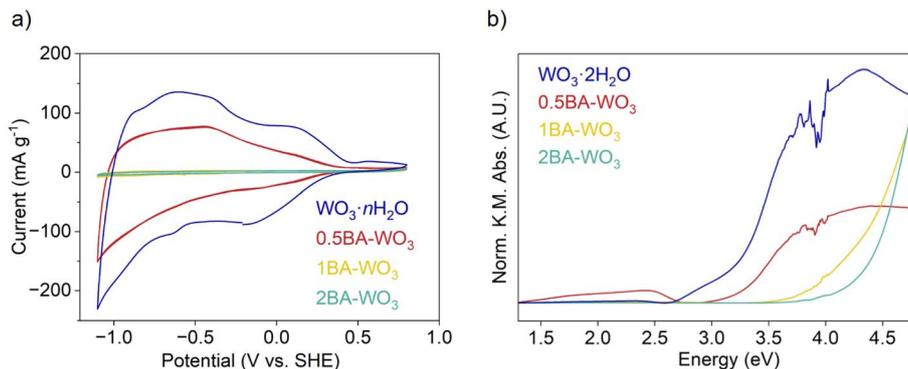
Fig. 3 (a) CVs of  $\text{WO}_3 \cdot n\text{H}_2\text{O}$  and butylammonium pillared tungsten oxides with various ratios in 0.1 M  $\text{LiClO}_4$  in PC at  $1 \text{ mV s}^{-1}$  (b) DRS of  $\text{WO}_3 \cdot 2\text{H}_2\text{O}$  and butylammonium pillared tungsten oxides with various ratios.
