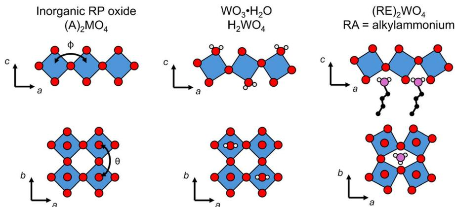
Fig. 4 Generic representation of the octahedral layers in an all-inorganic RP oxide,  $\text{WO}_3 \cdot \text{H}_2\text{O}$ , and a hybrid RP oxide. The two common types of tilting ( $\varphi$  and  $\theta$ ) are shown in the respective viewing orientation. Blue polyhedral, red spheres, grey spheres, and purple spheres represent W-centered octahedral units, oxygen atoms, hydrogen atoms, and nitrogen atoms, respectively.
