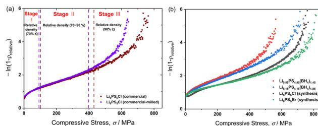
Fig. 2 (a) The Heckel plots of commercial  $\text{Li}_6\text{PS}_5\text{Cl}$  with that of the same powder after ball-milling (vibrating mill). The pressure required to reach each stage is different for each electrolyte. (b) The Heckel plots of various argyrodite solid electrolyte powders.
