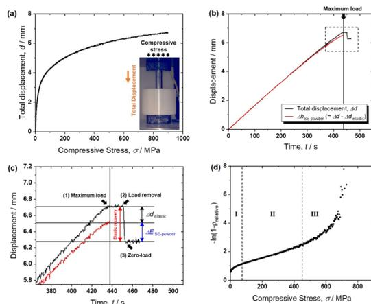
Fig. 1 (a) The total displacement ( $\Delta d$ ) curve corresponding to the compressive stress ( $\sigma$ ). (b)  $\Delta d$  and  $\Delta h_{\text{SE-powder}}$  with time for commercial  $\text{Li}_6\text{PS}_5\text{Cl}$  powder. (c) The magnified image of the dotted line square segment in (b). (d) The negative natural logarithmic ( $1 - \rho_{\text{relative}}$ ) vs. the compressive stress curve of the commercial  $\text{Li}_6\text{PS}_5\text{Cl}$  powder.
