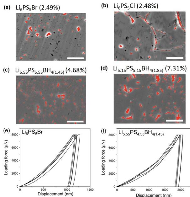
Fig. 3 (a–d) Porosity of cross-sections of different types of solid electrolyte pellets measured by SEM. The scale bar is 3  $\mu\text{m}$ . The black spot, which resembles a pore-like feature, is an artifact caused by the ‘edge effect,’ as explained in detail in Fig. S3.† (e and f) Indentation curve of a synthesized sample. Measurements were taken at least five times at different locations for each sample.
