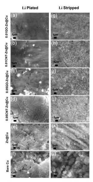
Fig. 4 SEM images of Li-plated electrodes; (a) 0.01GO-Zn@Cu; (b) 0.01CNT-Zn@Cu; (c) 0.05GO-Zn@Cu; (d) 0.05CNT-Zn@Cu; (e) Zn@Cu; (f) bare Cu. SEM images of Li-fully stripped electrodes; (g) 0.01GO-Zn@Cu; (h) 0.01CNT-Zn@Cu; (i) 0.05GO-Zn@Cu; (j) 0.05CNT-Zn@Cu; (k) Zn@Cu; (l) bare Cu.
