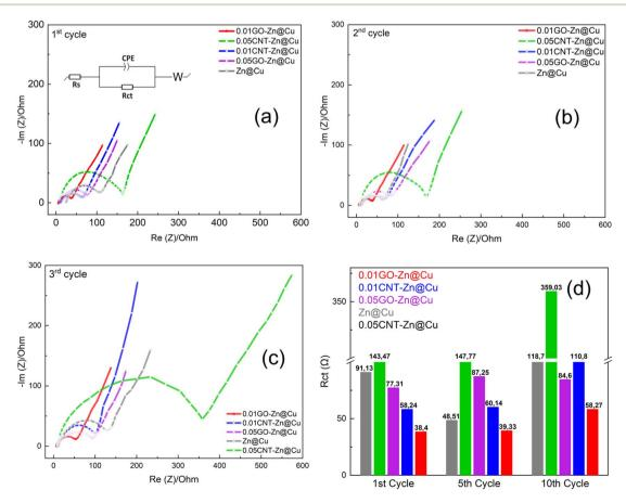
Fig. 8 EIS spectra of the half cells after being fully stripped at 1 V at different cycles. (a) After the 1st cycle (inset shows the equivalent circuit model of half-cells). (b) After the 5th cycle and (c) after the 10th cycle. (d) Reported charge transfer ( $R_{ct}$ ) values
