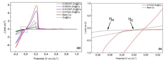
Fig. 3 (a). CV curves of the bare Cu foil, Zn@Cu, and composite coated electrodes at a scan rate of 0.5 mV s<sup>-1</sup>; (b) the inset indicates the onset of nucleation for bare Cu and 0.01GO-Zn@Cu electrodes.
