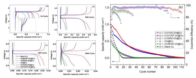
Fig. 9 (a) Voltage profiles of the anode-free LFP||modified-Cu full cell for different cycles; (a) 1st cycle and the inset shows a distinct new plateau around 3 V, indicating the transfer of active Li. (b) 20th cycle. (c) 40th cycle. (d) 100th cycle. (e) Extended cycling performance of the anode-free LFP||modified-Cu full cells indicating capacity retention and CE%.
