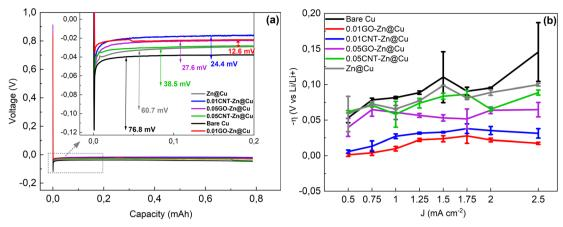
Fig. 6 (a) Half-cell discharge curves of all cells at 0.5 mA cm<sup>-2</sup>; the inset shows the Li nucleation region of the cells. (b) The Li nucleation overpotential for all cells at different current densities.
