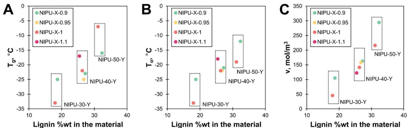
Fig. 10 Thermo-mechanical properties of NIPUs measured using DSC and DMA. (A) Glass transition temperatures ( $T_g$ ) based on DSC curves. (B) Alpha transition temperatures ( $T_\alpha$ ) based on DMA. (C) Crosslinking density of the network ( $\nu$ ) based on DMA. In all the graphs, "NIPU-X-1" represents all the NIPUs with a C/OH ratio of 1, and "NIPU-40-Y" represents all the NIPUs produced with L-pOH-40.
