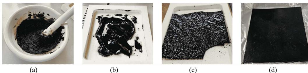
Fig. 9 Synthesis steps of NIPU-40-1. (a) Initial mixing of L-pOH and HMDC at room temperature. (b) Homogeneous reaction mixture before curing. (c) NIPU-40-1 after 3 h at 140 °C and 2 h at 160 °C. Trapped bubbles can be observed on the surface of the material. (d) Final product obtained after hot pressing at 160 °C for 30 min.
