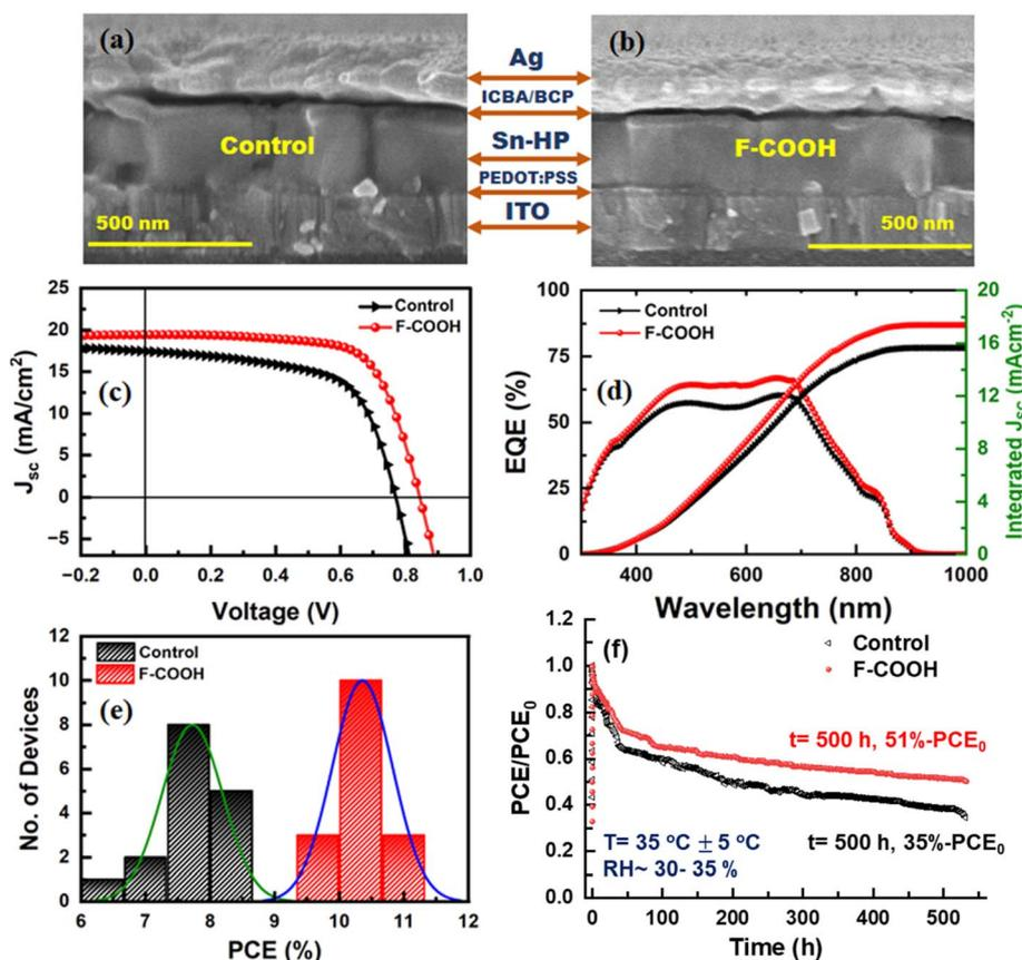
Fig. 2 Cross-sectional SEM images of devices (a) control and (b) with F-COOH additive. (c)  $J$ - $V$  curves of devices. (d) EQE spectra. (e) Statistical histogram of corresponding device efficiencies (16 devices from 4 batches). (f) Operational stability of Sn-PSCs under MPPT conditions and air ambient (ISOS-L-1).
