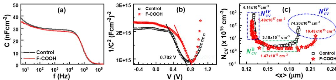
Fig. 5 Capacitance characteristics of devices: (a)  $C$ - $f$  spectra under darkness, (b) Mott-Schottky plots, (c) carrier profile of the device without and with F-COOH additive.
