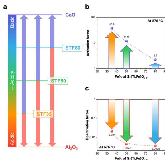
Fig. 4 Relative Smith acidity of  $\text{SrTi}_{1-x/100}\text{Fe}_{x/100}\text{O}_{3-\delta}$  (STF $x$ ,  $x = 35, 50, 80$ ) specimens and their infiltrates, along with trends in degree of activation. (a) Qualitative relative Smith acidity of the STF $x$  specimens, along with that of CaO, and  $\text{Al}_2\text{O}_3$ . (b) Activation factor in case of CaO infiltration (c) Deactivation factor in case of  $\text{Al}_2\text{O}_3$  infiltration.
