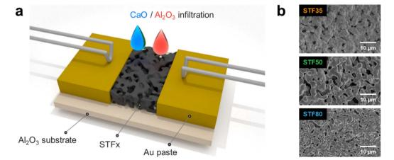
Fig. 1 Experimental set-up for measuring surface oxygen exchange coefficient,  $k_{\text{chem}}$  of porous specimens. (a) Schematic of DC conductivity relaxation measurement set-up and (b) surface morphology of  $SrTi_{1-x/100}Fe_{x/100}O_{3-\delta}$  samples (x=35,50,80).
