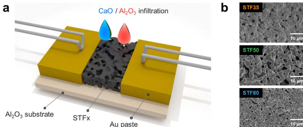
Fig. 1 Experimental set-up for measuring surface oxygen exchange coefficient,  $k_{\text{chem}}$  of porous specimens. (a) Schematic of DC conductivity relaxation measurement set-up and (b) surface morphology of SrTi<sub>1-x/100</sub>Fe<sub>x/100</sub>O<sub>3- $\delta$</sub>  samples ( $x = 35, 50, 80$ ).
