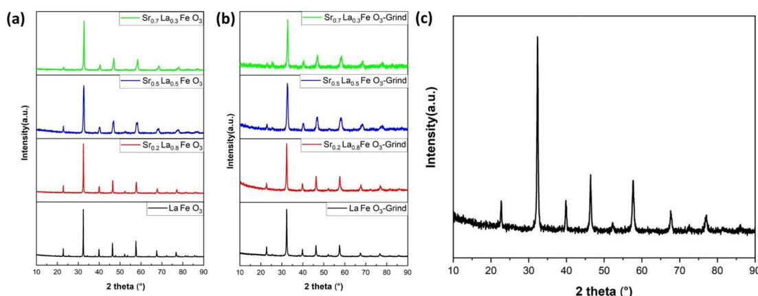
**Fig. 1** XRD results of Sr<sub>x</sub>La<sub>1-x</sub>FeO<sub>3</sub> ( $x = 0, 0.2, 0.5, 0.7$ ) perovskite oxide. (a) Before grinding with salt and (b) after grinding with salt. (c) XRD result of Sr<sub>0.2</sub>La<sub>0.8</sub>FeO<sub>3</sub> (electrospun).
