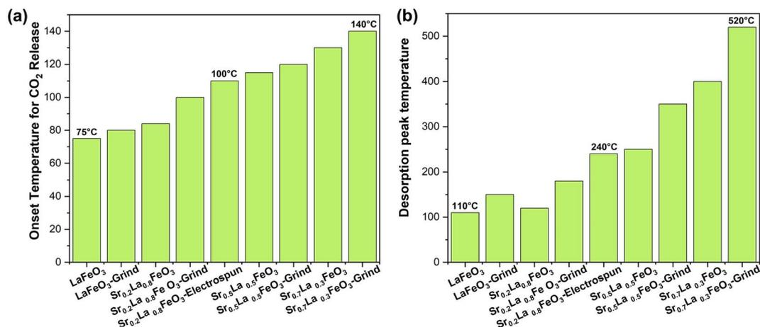
Fig. 2 TGA results of Sr<sub>x</sub>La<sub>1-x</sub>FeO<sub>3</sub> perovskite oxide. (a) Onset temperature for CO<sub>2</sub> release of Sr<sub>x</sub>La<sub>1-x</sub>FeO<sub>3</sub> perovskite oxide ( $x = 0, 0.2, 0.5, 0.7$ ). (b) Desorption peak temperature of Sr<sub>x</sub>La<sub>1-x</sub>FeO<sub>3</sub> perovskite oxide ( $x = 0, 0.2, 0.5, 0.7$ ).
