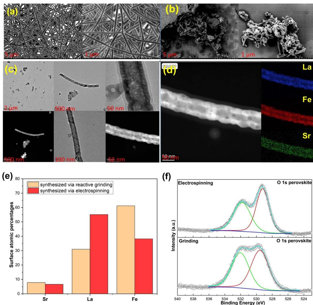
Fig. 4 (a) SEM image of  $\text{Sr}_{0.2}\text{La}_{0.8}\text{FeO}_3$  prepared by electrospinning before calcination; (b) post-calcination; (c) TEM images of the electrospun sample; (d) corresponding elemental mapping by EDS; (e) comparison of the XPS derived near surface atomic surface percentages between samples prepared via electrospinning and grinding methods; (f) comparisons of the O 1s spectra of the electrospun and reactive ground samples.
