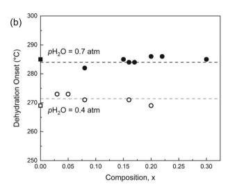
Fig. 6 Decomposition temperature of materials in the (1-x) CsH<sub>2</sub>PO<sub>4</sub>-xCs<sub>2</sub>HPO<sub>4</sub> system: (a) as a function of pH<sub>2</sub>O with x=0.1; and (b) as a function of composition, x, at pH<sub>2</sub>O values indicated.
