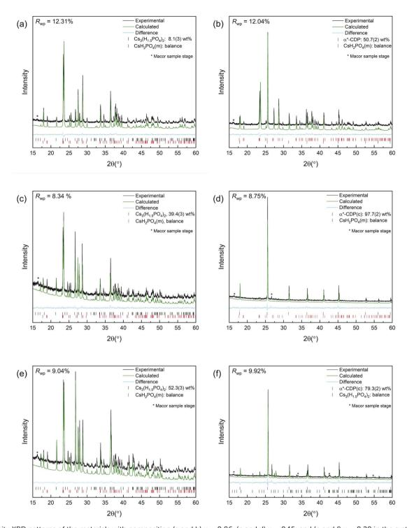
Fig. 2 In situ XRD patterns of the materials with composition (a and b) x = 0.06, (c and d) x = 0.15; and (e and f) x = 0.20 in the system (1 - x) $CsH_2PO_4 - xCs_2HPO_4$  at (a, c and e) 150 °C, below the eutectoid transition, and (b, d and f) 197 °C, above the transition. The composition x = 0.15is close to the eutectoid composition, and at 197 °C, almost all of the material has transformed to cubic  $\alpha$ -CPD. Data are collected under flowing  $pH_2O = 0.4$  atm, balance  $N_2$ .
