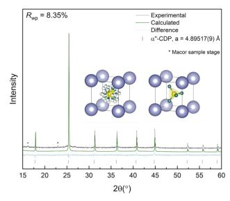
Fig. 7 Rietveld refinement result from measurement of the x=0.16 composition at 222 °C. Insets show the refined structure, corresponding to a stoichiometry of  $CsH_{1.59}(PO_4)_{0.86}$  with 14% of the phosphate sites unoccupied. Left inset is the average structure, with all oxygen sites shown; right inset displays a single representative phosphate orientation.
