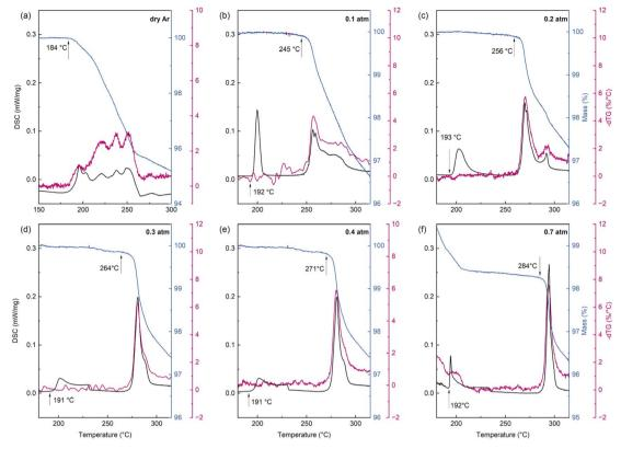
Fig. 5 STA profiles of the material with composition x = 0.16, close to the eutectoid composition, in the  $(1 - x)CsH_2PO_4 - xCs_2HPO_4$  system measured under six different gas conditions ranging from (a) dry Ar; to (f) 0.7 atm, as indicated. In the absence of humidification, the polymorphic transition is convoluted with decomposition. With increasing pH<sub>2</sub>O, the decomposition is increasingly suppressed.
