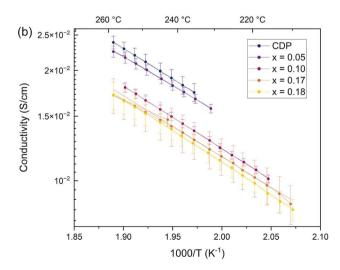
Fig. 8 Conductivities of representative materials in the (1 - x) $CsH_2PO_4-xCs_2HPO_4$  system collected under  $pH_2O=0.4$  atm: (a) Arrhenius presentation showing behavior over the temperature range 150-260 °C; and (b) behavior in the superprotonic phase space.
