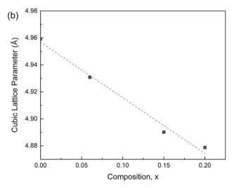
Fig. 3 Cubic lattice parameters of  $\alpha''$ -CDP materials: (a) temperature dependence, with filled data points corresponding to single phase regions and half-filled data points to single phase regions; and (b) composition dependence at 192 °C, where values are extrapolated from (a). The data for stoichiometric CDP (x=0) are from Ikeda *et al.*<sup>21</sup> Uncertainties in the values as derived from Rietveld refinement are smaller than the size of the datapoints.
