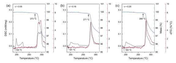
Fig. 4 STA profiles of representative materials in the (1-x)CsH<sub>2</sub>PO<sub>4</sub>-xCs<sub>2</sub>HPO<sub>4</sub> system collected under pH<sub>2</sub>O = 0.4 atm: (a) x = 0.05 (in the hypoeutectoid region); (b) x = 0.16 (close the eutectoid composition); and (c) x = 0.20 (in the hypereutectoid region). Each material displays a DSC anomaly at ~192 °C in the absence of mass loss.
