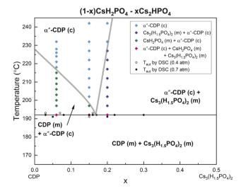
Fig. 1 Phase diagram between  $CsH_2PO_4$  and  $Cs_3(H_{1.5}PO_4)_2$  as determined from STA and *in situ* XRD experiments. For ease of description, the composition space is defined according to  $(1 - x)CsH_2PO_4 - xCs_2HPO_4$ .
