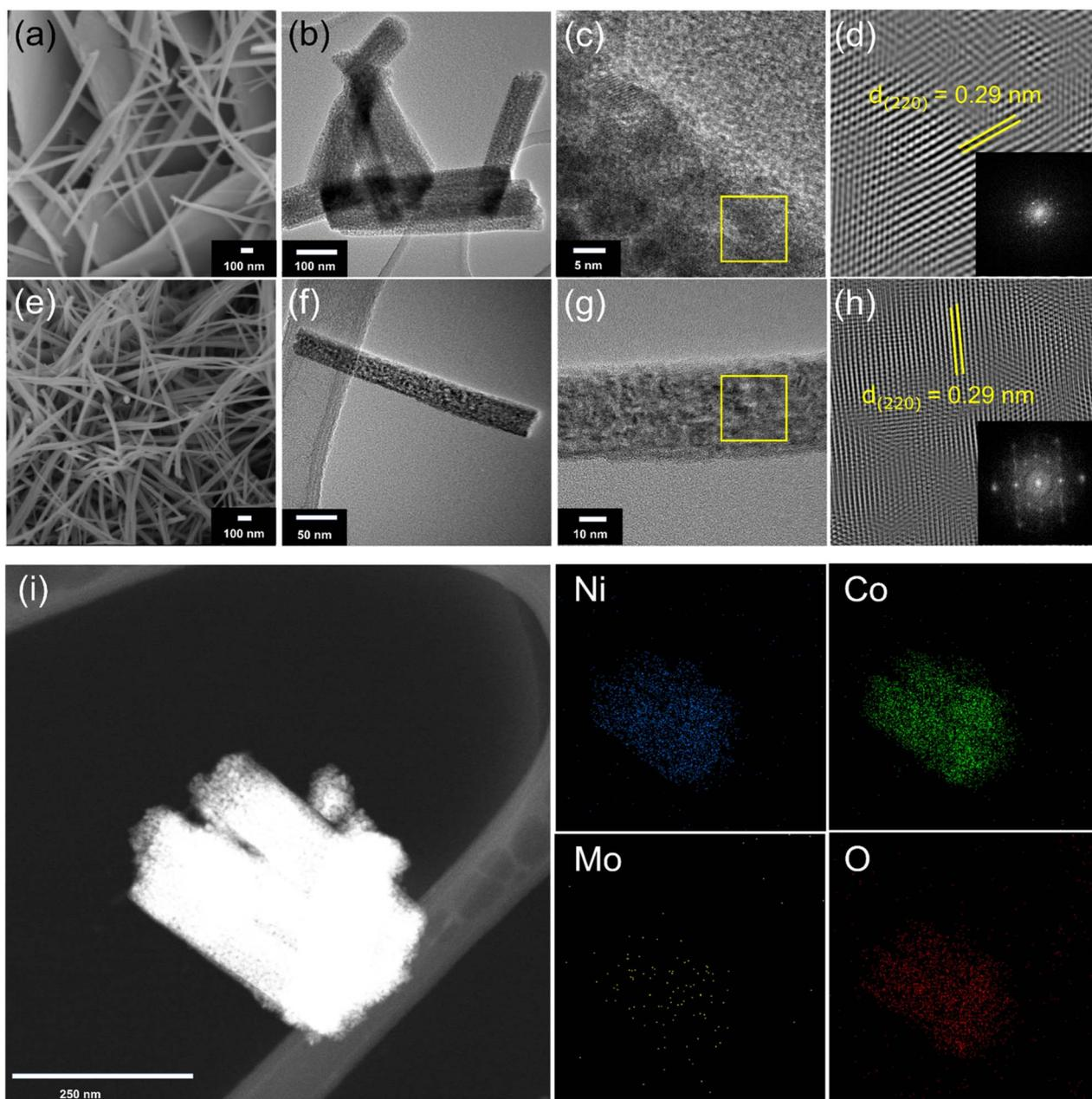
Fig. 2 (a and b) SEM and HR-TEM images of  $\text{NiCo}_2\text{O}_4$ . (c and d) HR-TEM of  $\text{NiCo}_2\text{O}_4$  showing the crystal lattice fringes. (e and f) SEM and HR-TEM images of  $\text{NiCo}_{1.9}\text{Mo}_{0.1}\text{O}_4$ . (g and h) HR-TEM of  $\text{NiCo}_{1.9}\text{Mo}_{0.1}\text{O}_4$  showing the crystal lattice fringes. (i) EDS atomic elemental mapping of trimetallic  $\text{NiCo}_{1.9}\text{Mo}_{0.1}\text{O}_4$ .
