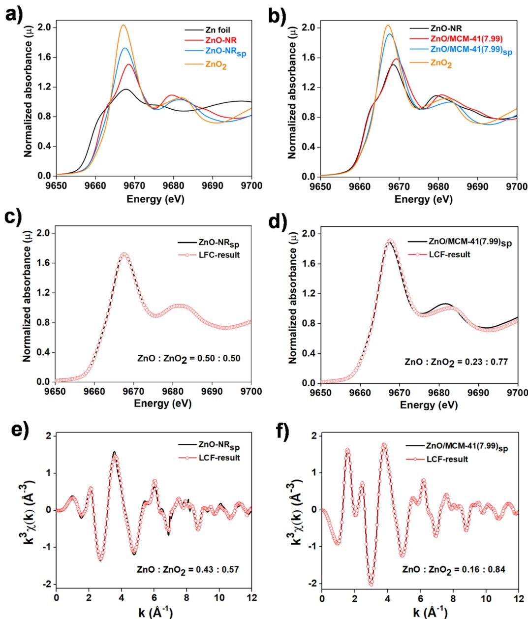
Fig. 6 (a and b) Normalized Zn K-edge XANES spectra of Zn foil, ZnO-NR, ZnO-NR<sub>sp</sub>, ZnO/MCM-41(7.99), ZnO/MCM-41(7.99)<sub>sp</sub>, and ZnO<sub>2</sub> NPs. (c and d) LCF results for the Zn K-edge XANES of the spent catalysts. (e and f) LCF results for the  $k^3$ -weighted EXAFS data of the spent catalysts.
