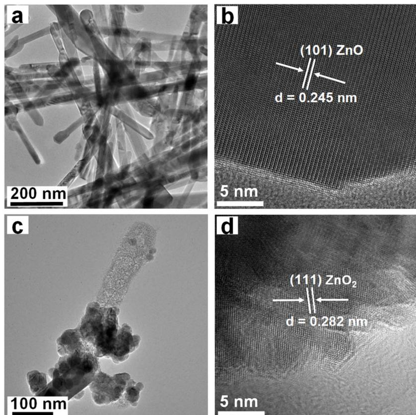
Fig. 4 TEM (a and c) and HRTEM (b and d) images of ZnO-NR (a and b) and ZnO-NR<sub>sp</sub> (c and d).
