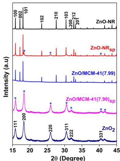
Fig. 3 SXR D patterns of ZnO-NR, ZnO-NR<sub>sp</sub>, ZnO/MCM-41(7.99), ZnO/MCM-41(7.99)<sub>sp</sub>, and ZnO<sub>2</sub> NPs (X-ray wavelength of 0.77489 Å). The peaks marked by asterisks are attributed to cubic ZnO<sub>2</sub>.
