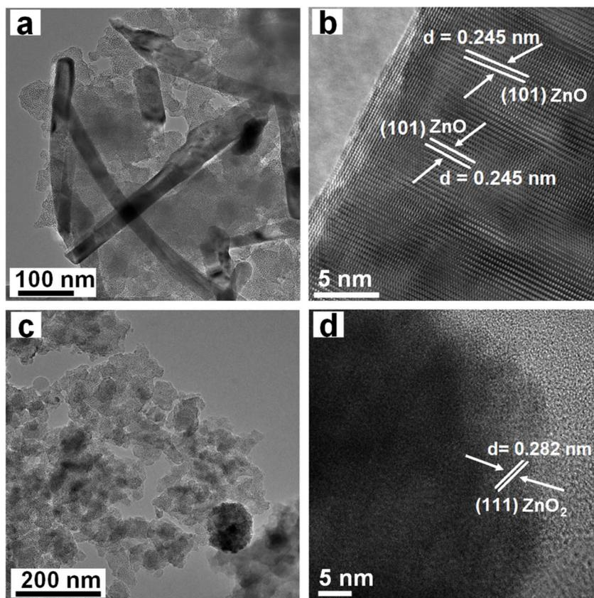
Fig. 5 TEM (a and c) and HRTEM (b and d) images of ZnO/MCM-41(7.99) (a and b) and ZnO/MCM-41(7.99)<sub>sp</sub> (c and d).
