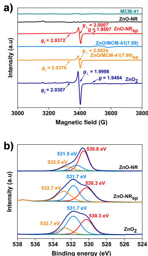
Fig. 8 (a) EPR spectra of MCM-41, ZnO-NR, ZnO-NR<sub>sp</sub>, ZnO/MCM-41(7.99), ZnO/MCM-41(7.99)<sub>sp</sub>, and  $\text{ZnO}_2$  NPs measured at 77 K. (b) O 1s XPS spectra and deconvoluted peaks of ZnO-NR, ZnO-NR<sub>sp</sub>, and  $\text{ZnO}_2$  NPs.
