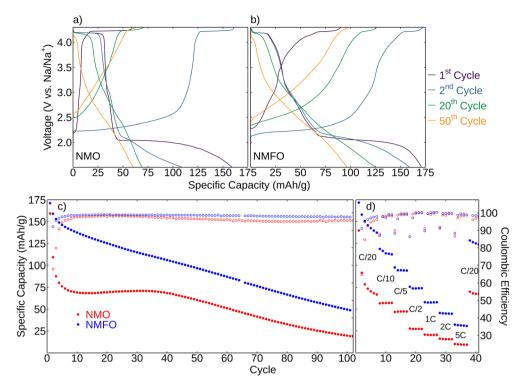
Fig. 6 Electrochemical testing of  $Na_2Mn_3O_7$  (NMO) and  $Na_{2.25}Mn_{2.75}Fe_{0.25}O_7$  (NMFO) over the voltage range 1.5–4.3 V vs. Na/Na<sup>+</sup>. Select voltage profiles of (a) NMO and (b) NMFO cycled at C/20. (c) Cycling performance at C/20 with specific capacity (left axis, filled points) and coulombic efficiency (right axis, empty points) as a function of cycle. (d) Rate performance evaluation.
