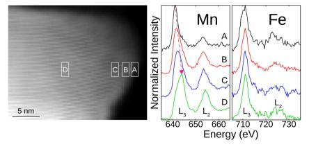
Fig. 2 EELS measurements for Na<sub>2.25</sub>Mn<sub>2.75</sub>Fe<sub>0.25</sub>O<sub>7</sub>. The particle on which these measurements are taken is shown on the left with the white boxes indicating the areas of the particle on which the measurements were taken moving from the edge of the particle (A) to the bulk (D). The associated EELS spectra are shown on the right, and the Mn and Fe L-edges are labeled. The pink arrow indicates the shift in Mn L<sub>3</sub>-edge.
