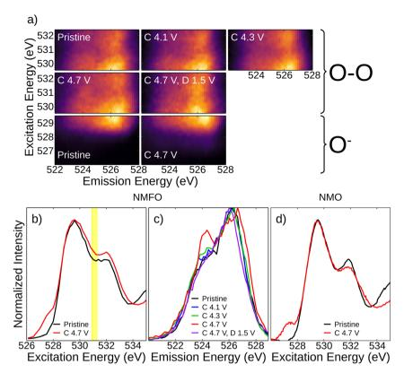
Fig. 5 Oxygen redox in Na<sub>2.25</sub>Mn<sub>2.75</sub>Fe<sub>0.25</sub>O<sub>7</sub> (NMFO) at different states of charge. (a) O K-edge RIXS maps of NMFO at different states of charge. (b) O K-edge XAS (via integration of RIXS maps) for NMFO pristine and fully charged. (c) Emission spectra for the region corresponding to excitation energies of 530.9-531.3 eV, highlighted in yellow in (b). (d) O K-edge XAS of  $Na_2Mn_3O_7$  at the same voltages as (b).
