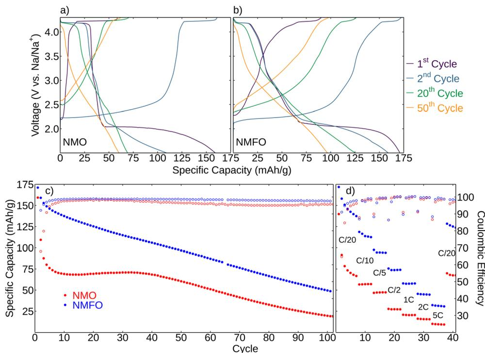
Fig. 6 Electrochemical testing of  $\text{Na}_2\text{Mn}_3\text{O}_7$  (NMO) and  $\text{Na}_{2.25}\text{Mn}_{2.75}\text{Fe}_{0.25}\text{O}_7$  (NMFO) over the voltage range 1.5–4.3 V vs.  $\text{Na}/\text{Na}^+$ . Select voltage profiles of (a) NMO and (b) NMFO cycled at C/20. (c) Cycling performance at C/20 with specific capacity (left axis, filled points) and coulombic efficiency (right axis, empty points) as a function of cycle. (d) Rate performance evaluation.
