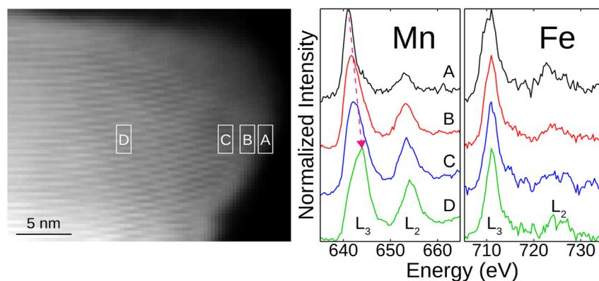
**Fig. 2** EELS measurements for  $\text{Na}_{2.25}\text{Mn}_{2.75}\text{Fe}_{0.25}\text{O}_7$ . The particle on which these measurements are taken is shown on the left with the white boxes indicating the areas of the particle on which the measurements were taken moving from the edge of the particle (A) to the bulk (D). The associated EELS spectra are shown on the right, and the Mn and Fe L-edges are labeled. The pink arrow indicates the shift in Mn  $L_3$ -edge.
