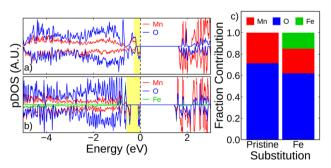
Fig. 3 Projected density of states (pDOS) for (a) Na<sub>2</sub>Mn<sub>3</sub>O<sub>7</sub> (NMO) and (b)  $Na_{2.5}Mn_{2.5}Fe_{0.5}O_7$  (NMFO). The yellow box highlights the area corresponding to the removal of one electron per formula unit, representing the amount of electrons estimated to be removed in the electrochemical voltage window shown later. (c) Fractional contributions of each element for pristine NMO and NMFO from the highlighted region in (a and b).
