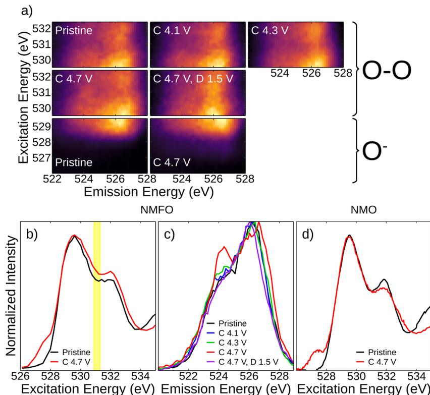
Fig. 5 Oxygen redox in  $\text{Na}_{2.25}\text{Mn}_{2.75}\text{Fe}_{0.25}\text{O}_7$  (NMFO) at different states of charge. (a) O K-edge RIXS maps of NMFO at different states of charge. (b) O K-edge XAS (via integration of RIXS maps) for NMFO pristine and fully charged. (c) Emission spectra for the region corresponding to excitation energies of 530.9–531.3 eV, highlighted in yellow in (b). (d) O K-edge XAS of  $\text{Na}_2\text{Mn}_3\text{O}_7$  at the same voltages as (b).
