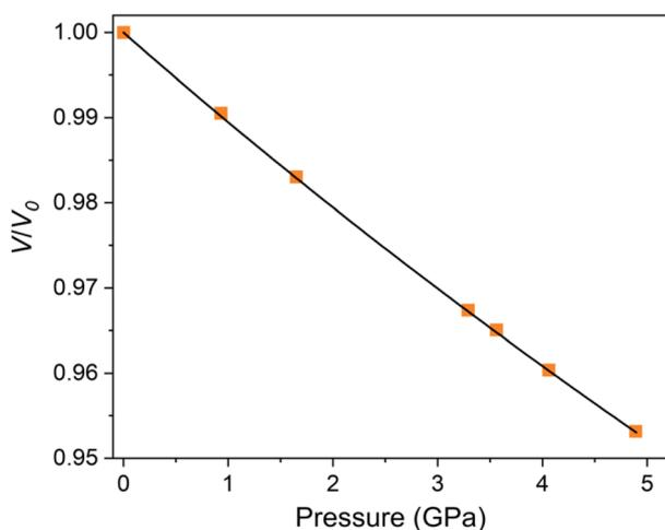
Fig. 3 Variation of normalised unit cell volume with pressure for  $\text{Ba}_7\text{Nb}_4\text{MoO}_{20}$ . The data is fit with a second order Birch–Murnaghan equation of state.
