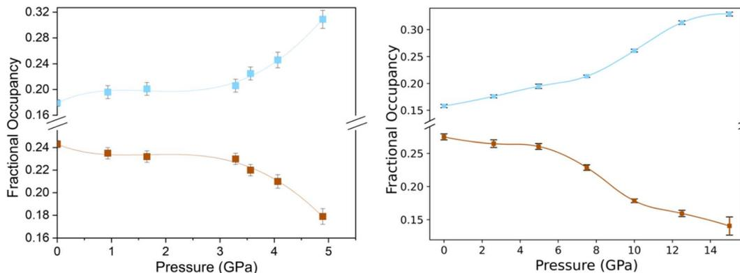
Fig. 4 Influence of pressure on O1 (orange) and O2 (blue) fractional occupancies from the Rietveld fit to the  $P\bar{3}m1$  model from neutron diffraction data collected on the PEARL diffractometer (left) and MD simulations at 300 K (right).
