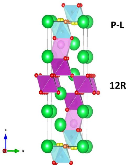
Fig. 1 Average crystal structure of  $\text{Ba}_7\text{Nb}_4\text{MoO}_{20}$  which is composed of alternating 12R perovskite and palmierite-like (P-L) layers. Colours: green, Ba; blue, M1; pink, M2; purple, M3 and M4; yellow, O1; orange, O2; and red, O3, O4, and O5. The O1 and O2 sites are partially occupied resulting in variable coordination of the M1 cations along the P-L layers.
