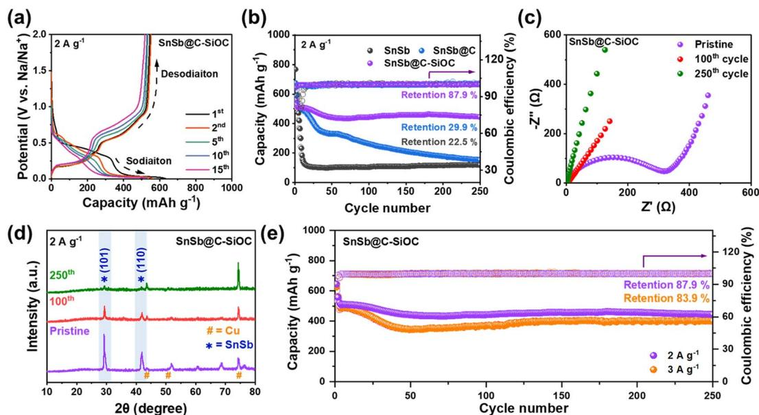
Fig. 4 (a) GCD profiles of the SnSb@C-SiOC nano-hybrid cell after several cycles (1st, 2nd, 5th, 10th, and 15th). (b) Cycling performance of SnSb, SnSb@C, and SnSb@C-SiOC at 2.0 A g<sup>-1</sup>, (c) Nyquist plots, and (d) *ex situ* XRD patterns of the SnSb@C-SiOC electrode obtained before cycling and after the 100th and 250th cycles. (e) High rate cycling performance of the SnSb@C-SiOC electrode at current densities of 2.0 and 3.0 A g<sup>-1</sup>.
