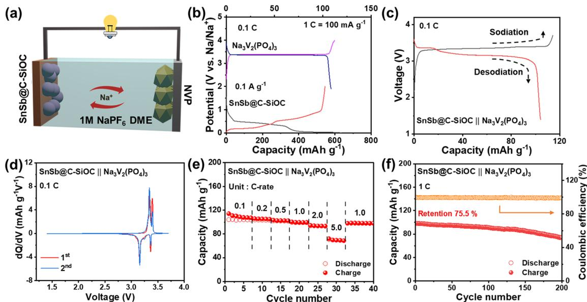
Fig. 7 (a) Schematic of the full cell configuration comprising the SnSb@C-SiOC anode and  $\text{Na}_3\text{V}_2(\text{PO}_4)_3/\text{C}$  (NVP) cathode. (b) GCD profiles of the NVP and SnSb@C-SiOC electrodes. (c) GCD profiles of the full cell at 0.1C. (d)  $dQ/dV$  plots for the 1st and 2nd cycles of the full cell at 0.1C. (e) Rate performance of the full cell at various C-rates from 0.1 to 5.0C. (f) Cycling performance of the full cell at 1.0C for 200 cycles.
