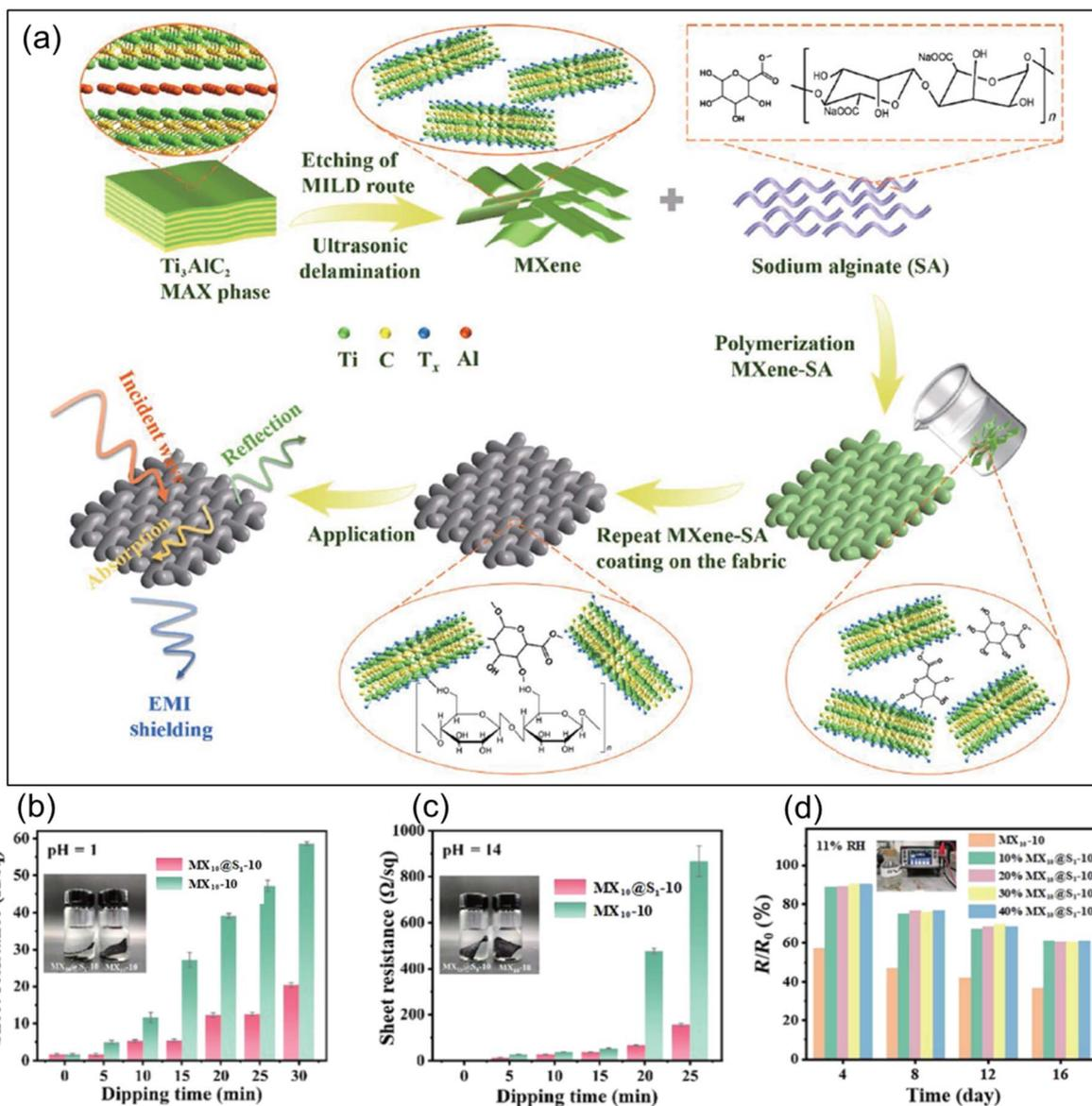
Fig. 6 (a) Schematic synthesis of MXene and illustration of the single-step fabrication strategy for sodium alginate–MXene films. Sheet-resistance ( $R/R_0$ ) variation upon treating in (b) HCl (pH = 1) and (c) NaOH (pH = 14), and (d) change in  $R/R_0$  for MX<sub>10</sub>-10 and MX<sub>10</sub>@S<sub>1</sub>-10 with varying SA content at 11% RH and 25 °C. Reproduced with permission from ref. 150. Copyright 2024, Springer Nature.
