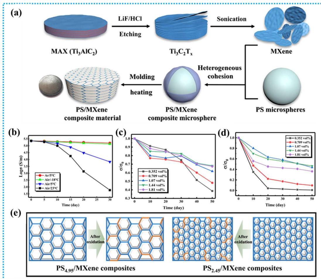
Fig. 4 (a) Schematic showing the exfoliation of  $\text{Ti}_3\text{C}_2\text{T}_x$  MXene and fabrication of composites with a three-dimensional conductive network framework, (b) storage environment effects on MXene's intrinsic conductivity. (c and d) Impact of environmental factors on conductivity during composite material preparation, and (e) schematic of the oxidation mechanism in the MXene-polymer composite. Reproduced with permission from ref. 140. Copyright 2021, Elsevier Ltd.
