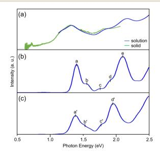
Fig. 2 (a) Optical absorbance (blue) and diffused reflectance (green) spectra of  $[Pt_{17}(CO)_{12}(PPh_3)_8]^z$  (z = 1+, 2+), and the calculated absorption spectra of (b)  $[Pt_{17}(CO)_{12}(P(CH_3)_3)_8]^{2+}$  $[Pt_{17}(CO)_{12}(PPh_3)_8]^{2+}$
