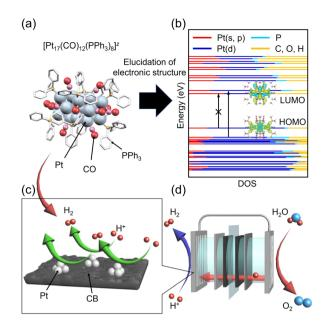
Fig. 1 Schematic of the work performed in this study. (a) Geometric and (b) calculated electronic structure of  $[Pt_{17}(CO)_{12}(PPh_3)_8]^z$  and its catalytic application to the (c) HER for (d) water electrolysis.
