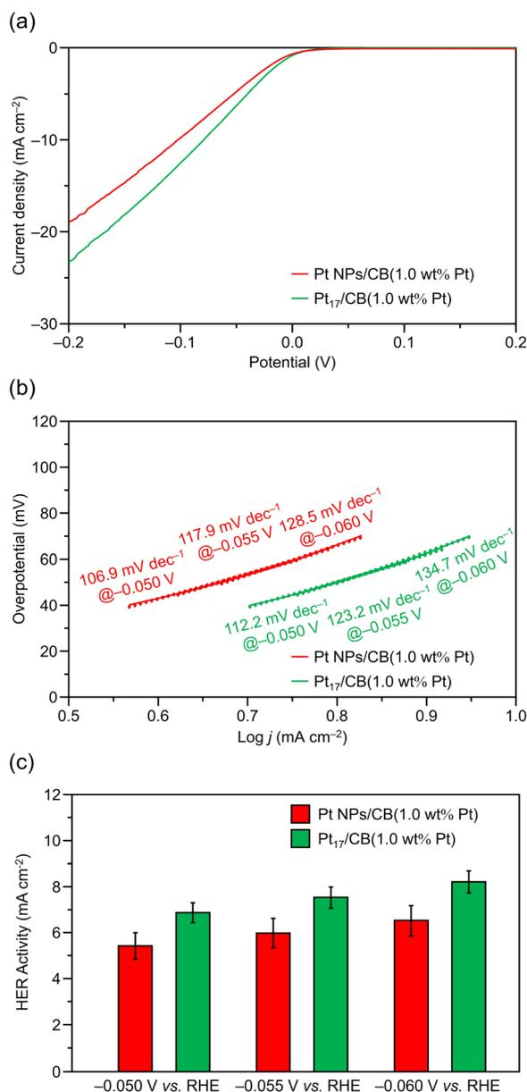
Fig. 6 (a) Representative LSV curves. (b) Tafel slopes and (c) HER activity of Pt<sub>17</sub>/CB(1.0 wt% Pt) and Pt NPs/CB(1.0 wt% Pt). For (b) and (c), data obtained at  $-0.050$ ,  $-0.055$ , and  $-0.060$  V vs. RHE are also shown for comparison.
