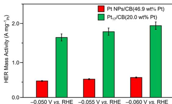
Fig. 7 HER mass activity of Pt<sub>17</sub>/CB(20.0 wt% Pt) and Pt NPs/CB(46.9 wt% Pt) obtained from the LSVs in Fig. S11.† Data obtained at  $-0.050$ ,  $-0.055$ , and  $-0.060$  V vs. RHE are also shown for comparison.
