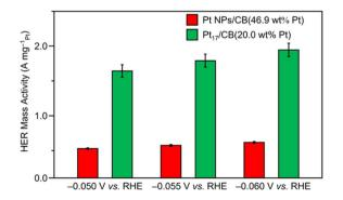
Fig. 7 HER mass activity of  $Pt_{17}/CB(20.0 \text{ wt}\% \text{ Pt})$  and Pt NPs/CB(46.9 wt% Pt) obtained from the LSVs in Fig. S11.† Data obtained at -0.050, -0.055, and -0.060 V vs. RHE are also shown for comparison.
