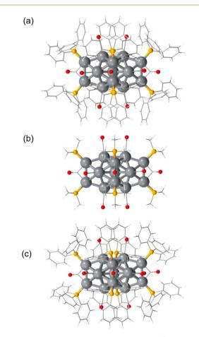
Fig. 3 Geometric structure of (a)  $[Pt_{17}(CO)_{12}(PPh_3)_8]^{2+}$  determined by SC-XRD from ref. 11 and the calculated most stable structures of (b)  $[Pt_{17}(CO)_{12}(P(CH_3)_3)_8]^{2+}$  and (c)  $[Pt_{17}(CO)_{12}(PPh_3)_8]^{2+}$ . Hydrogen and solvent atoms are omitted for clarity. Pt: grey, P: yellow, O: red, and carbon: light grey.
