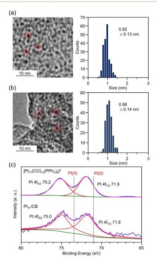
Fig. 5 TEM images and resulting histograms of particle-size distribution for (a)  $[Pt_{17}(CO)_{12}(PPh_3)_8]^z$  and (b)  $Pt_{17}/CB(1.0 \text{ wt% Pt})$ . (c)  $Pt 4f_{7/2}$ XPS spectra (blue line) and their fitting results (red, green, and magenta lines) for  $[Pt_{17}(CO)_{12}(PPh_3)_8]^z$  and  $Pt_{17}/CB(1.0 \text{ wt% Pt})$ . In (c), grey vertical lines indicate the position of Pt(0) and Pt(11).
