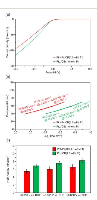
Fig. 6 (a) Representative LSV curves. (b) Tafel slopes and (c) HER activity of  $Pt_{17}/CB(1.0 \text{ wt}\% \text{ Pt})$  and Pt NPs/CB(1.0 wt% Pt). For (b) and (c), data obtained at -0.050, -0.055, and -0.060 V vs. RHE are also shown for comparison.
