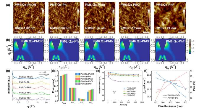
Fig. 4 (a) AFM images, (b) 2D GIWAXS patterns, and (c) out-of-plane and in-plane GIWAXS profiles for the five NFAs-based blend films. (d) Schematic of the energy loss and radiative and nonradiative recombination losses for devices. (e) Thermal stability of the devices. (f) J<sub>SC</sub> and PCE values of PM6:Qx-PhBr- and PM6:L8-BO-based devices with different thicknesses
