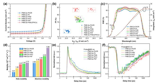
Fig. 3 (a) J-V curves, (b) FF and  $V_{\rm OC} imes J_{\rm SC}$  values distribution scatter chart, and (c) EQE curves of the devices. (d) Histograms of the hole and electron mobility of the blend films. Transient kinetic traces probed at (e) 880 nm and (f) 630 nm for the blend films.
