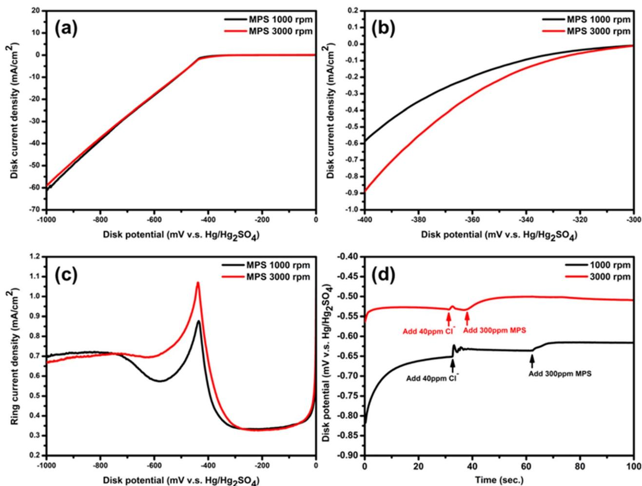
Fig. 2 (a and b) The RRDE study for (a) the LSVs of the disk electrode and (b) the enlarged curves of (a) from  $-300$  mV to  $-400$  mV and (c) the corresponding ring current against the disk electrode potential. (d) The chronopotentiograms measured at  $18 \text{ mA cm}^{-2}$  with chloride ions and MPS addition.
