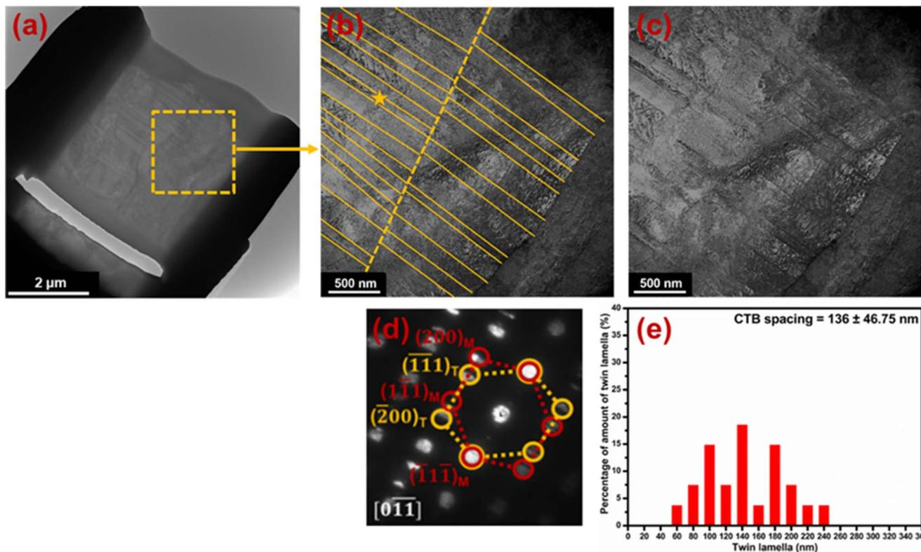
Fig. 6 TEM bright-field images of Cu plated at  $0.5 \text{ L} \cdot \text{min}^{-1}$  for (a) the entire copper sheet, and the HRTEM images within the yellow-bordered region shown in (b) with annotation lines (solid lines refer to twin boundaries and dashed lines refer to grain boundaries) and in (c) without annotations. (d) The SAED image taken at the star-marked location in (b). (e) The twin distribution identified within the same region.
