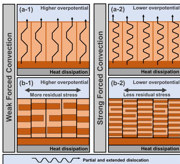
Fig. 10 The schemes of forming (a) the partial and extended dislocations and (b) the nanotwinned structure by electroplating at the aeration flow rates of (1) 0.5 L·min<sup>-1</sup> and (2) 2.5 L·min<sup>-1</sup>.
