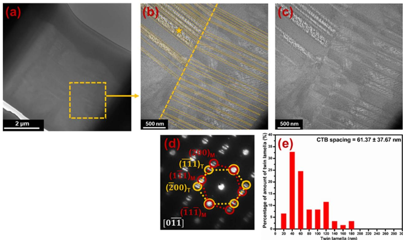
Fig. 7 TEM bright-field images of Cu plated at  $2.5 \text{ L} \cdot \text{min}^{-1}$  for (a) the entire copper sheet with the HRTEM images within the yellow-bordered region shown in (b) with annotation lines (solid lines refer to twin boundaries and dashed lines refer to grain boundaries) and in (c) without annotations. (d) The SAED image taken at the star-marked location in (b). (e) The twin distribution identified within the same region.
