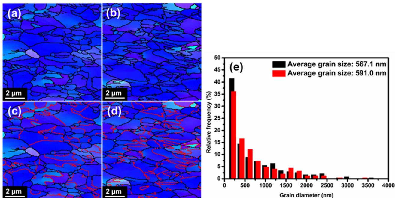
Fig. 4 The EBSD images of copper foil prepared at the aeration flow rates of (a and c)  $0.5 \text{ L} \cdot \text{min}^{-1}$  and (b and d)  $2.5 \text{ L} \cdot \text{min}^{-1}$  with the red line marks of (111) nanotwin in (c and d). (e) The grain sizes of copper foil prepared at the aeration flow rates of  $0.5 \text{ L} \cdot \text{min}^{-1}$  (black bar) and  $2.5 \text{ L} \cdot \text{min}^{-1}$  (red bar).
