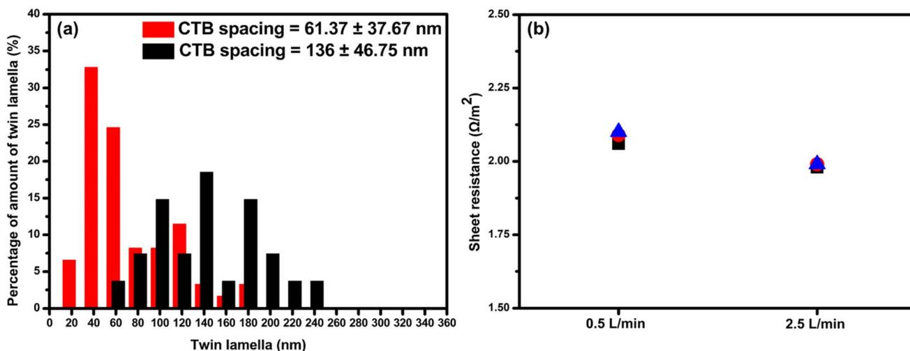
Fig. 8 (a) The distributions of twin spacing collected from the bright field HRTEM images and (b) the sheet resistance of the Cu foil electroplated at the aeration flow rates of (black bars)  $0.5 \text{ L} \cdot \text{min}^{-1}$  and (red bars)  $2.5 \text{ L} \cdot \text{min}^{-1}$ .
