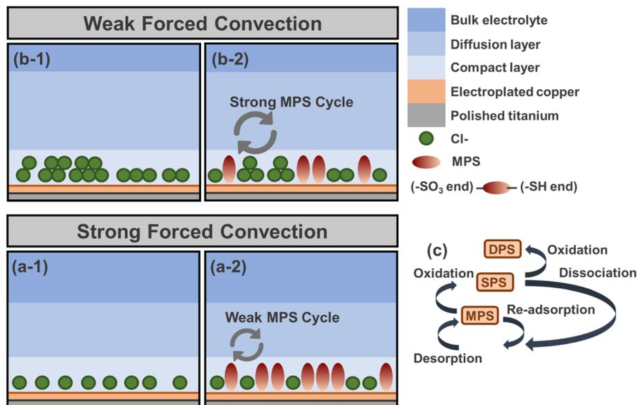
Fig. 9 The schemes of (a) merely Cl<sup>-</sup> and (b) Cl<sup>-</sup>/MPS adsorption near the cathode by electroplating at the aeration flow rates of (1) 0.5 L·min<sup>-1</sup> and (2) 2.5 L·min<sup>-1</sup>. (c) The details of the MPS cycle.
