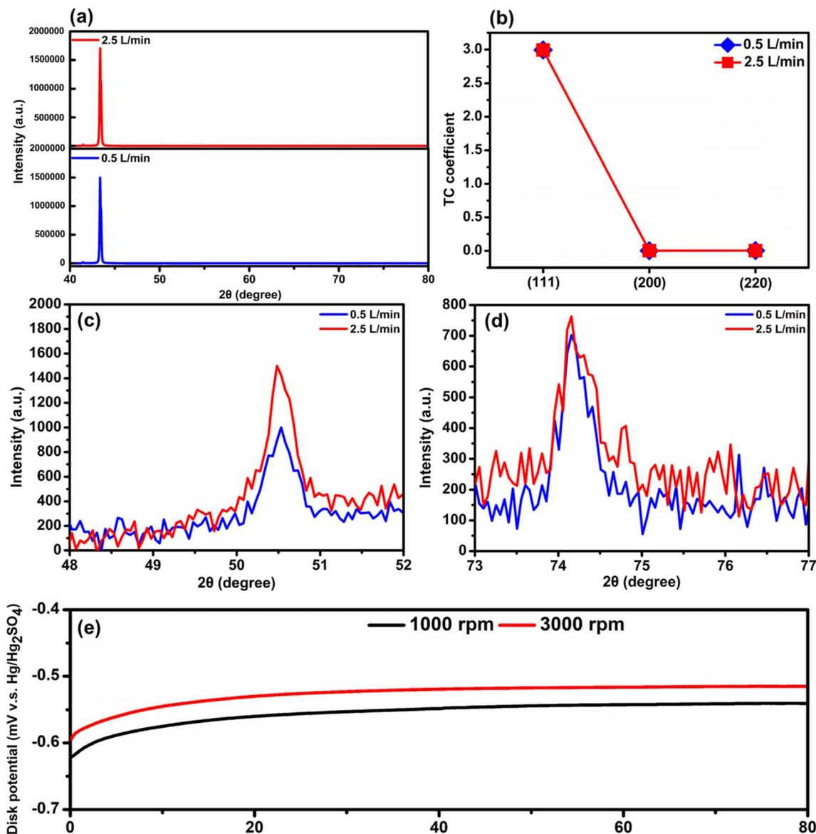
Fig. 3 (a) The XRD patterns and (b) the texture coefficient values of Cu plated at 40 ASD at the aeration flow rates of 0.5 and 2.5 L·min<sup>-1</sup> in the VMS added with 40 ppm chloride ions and 300 ppm MPS; the enlarged XRD images (c) from 48° to 52° and (d) from 73° to 77°. (e) The chronoamperograms of disk electrodes at 1000 and 3000 rpm in the VMS added with 40 ppm chloride ions and 300 ppm MPS at 18 mA·cm<sup>-2</sup>.
