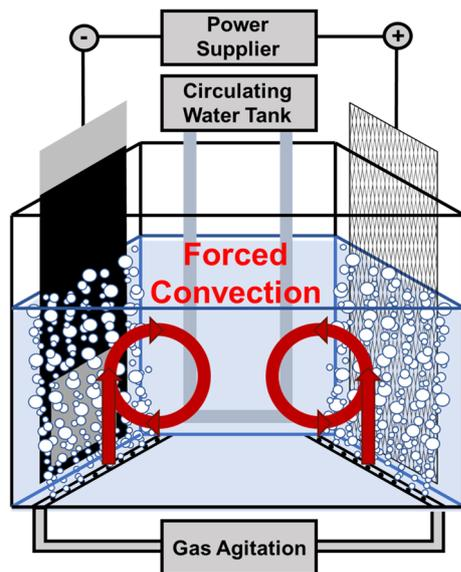
Fig. 1 The schematic of the copper electroplating apparatus.
