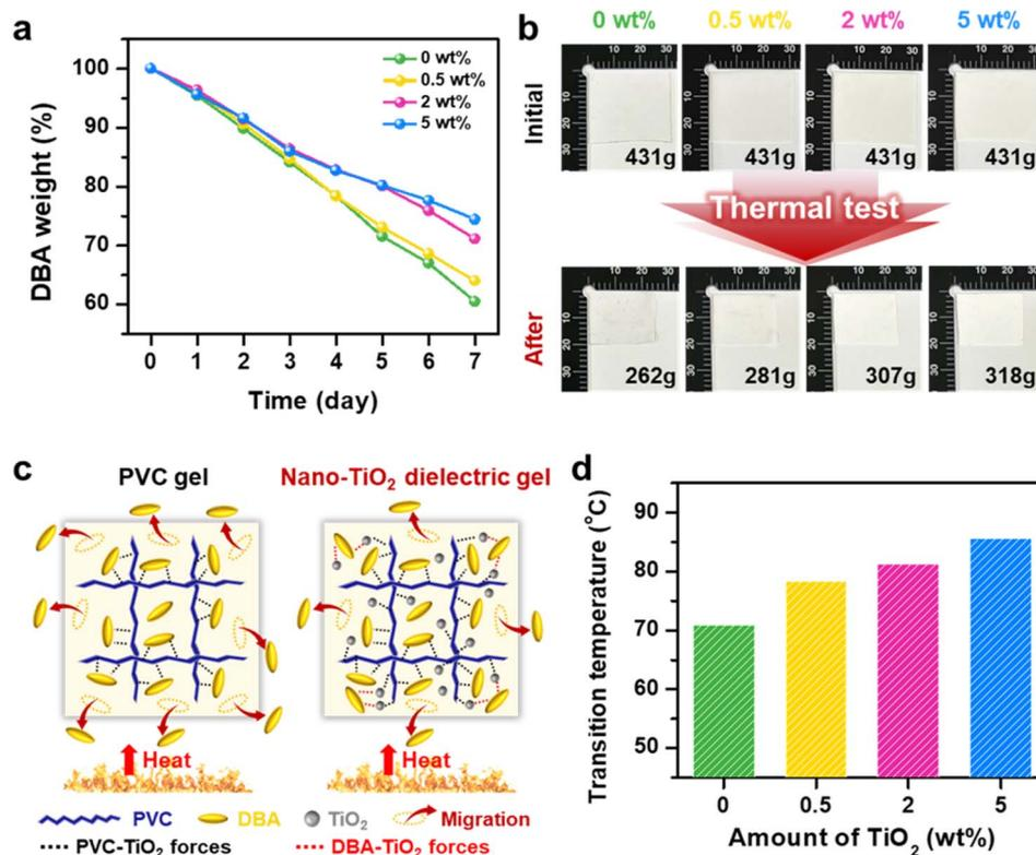
Fig. 5 Long term thermal stability of PVC gel and TiO<sub>2</sub> dielectric gels. (a) DBA weight change of PVC gel and TiO<sub>2</sub> dielectric gels over time at 60 °C. (b) Photographs of PVC gel and TiO<sub>2</sub> dielectric gels before and after 7 days thermal test at 60 °C. (c) Schematic of DBA plasticizer migration to the air by heat energy. (d) DSC transition temperature of PVC gel and TiO<sub>2</sub> dielectric gels.
