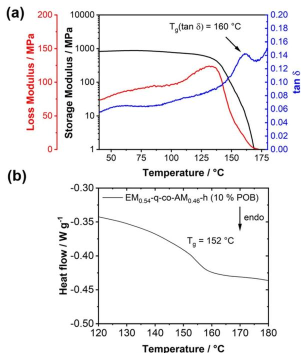
Fig. 6 (a) Dynamic mechanical analysis of  $\text{EM}_{0.54}\text{-q-co-AM}_{0.46}\text{-h}$  revealing only one glass transition temperature (2 K  $\text{min}^{-1}$  heating rate, 1 Hz oscillation frequency). (b) DSC analysis (2nd heating curve, 10 K  $\text{min}^{-1}$  heating rate) of a blend membrane consisting of 90 wt%  $\text{EM}_{0.54}\text{-q-co-AM}_{0.46}\text{-h}$  and 10 wt% POB.
