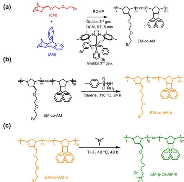
Fig. 1 (a) Synthesis of the precursor polymer (EM-co-AM) via ROMP utilizing the 3rd generation Grubbs catalyst with a 54 : 46 molar ratio of EM/AM in the feed (IEC<sub>theo</sub> = 2.00 mmol g<sup>-1</sup>). (b) Hydrogenation of the double bonds with *p*-toluenesulfonyl hydrazide. (c) Quaternization with trimethylamine.
