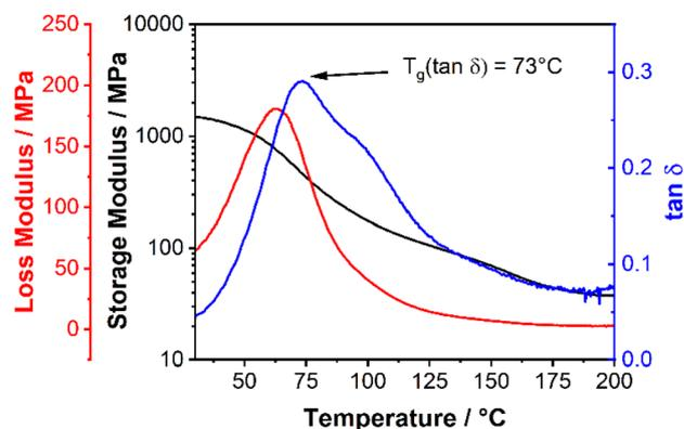
Fig. 4 Dynamic mechanical analysis (2 K min<sup>-1</sup> heating rate, 1 Hz oscillation frequency) of EM<sub>0.54</sub>-q-block-AM<sub>0.46</sub>-h revealing only one glass transition temperature.
