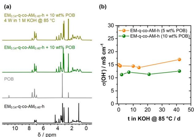
Fig. 8 (a) <sup>1</sup>H NMR spectra of the pure EM<sub>0.54</sub>-q-co-AM<sub>0.46</sub>-h (black), pure POB (grey) the pristine blend consisting of 10 wt% POB and 90 wt% EM<sub>0.54</sub>-q-co-AM<sub>0.46</sub>-h (green) and after treating the respective membrane with 1 M KOH at 85 °C for 4 weeks (yellow). (b) Ionic conductivity after certain time intervals in 1 M KOH at 85 °C.
