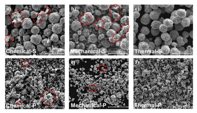
Fig. 4 SEM images of LNMO-S (top) and LNMO-P (bottom) particle materials recovered by chemical (left), mechanical (center), and thermal (right) separation techniques. Red circles mark the presence of undesired residuals.
