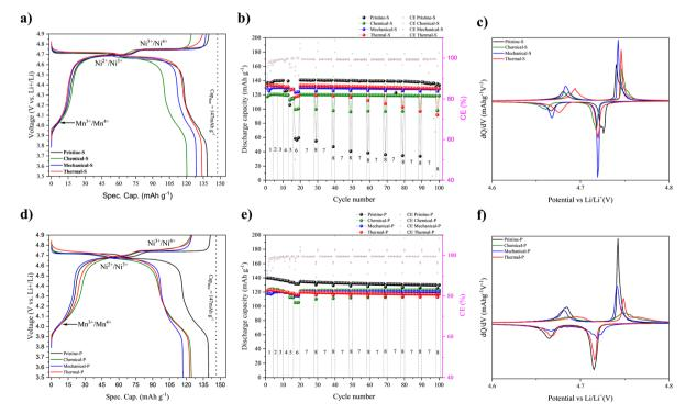
Fig. 7 (Left) Voltage profile of the third cycle, center: capacity and coulombic efficiency, and right  $\delta Q/\delta V$  for the LNMO-S (top) and LNMO-P (bottom) samples. The black, green, blue, and red (from bottom to top) correspond to the base pristine and compared chemical, mechanical, and thermal recovered samples respectively.
