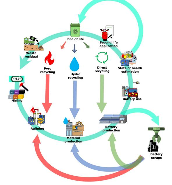
Fig. 1 Lithium-ion battery life cycle and the principal recycling routes depicting the origin of two main sources of recyclable materials; i.e. from end-of-life batteries (top) and from battery production scraps (bottom).
