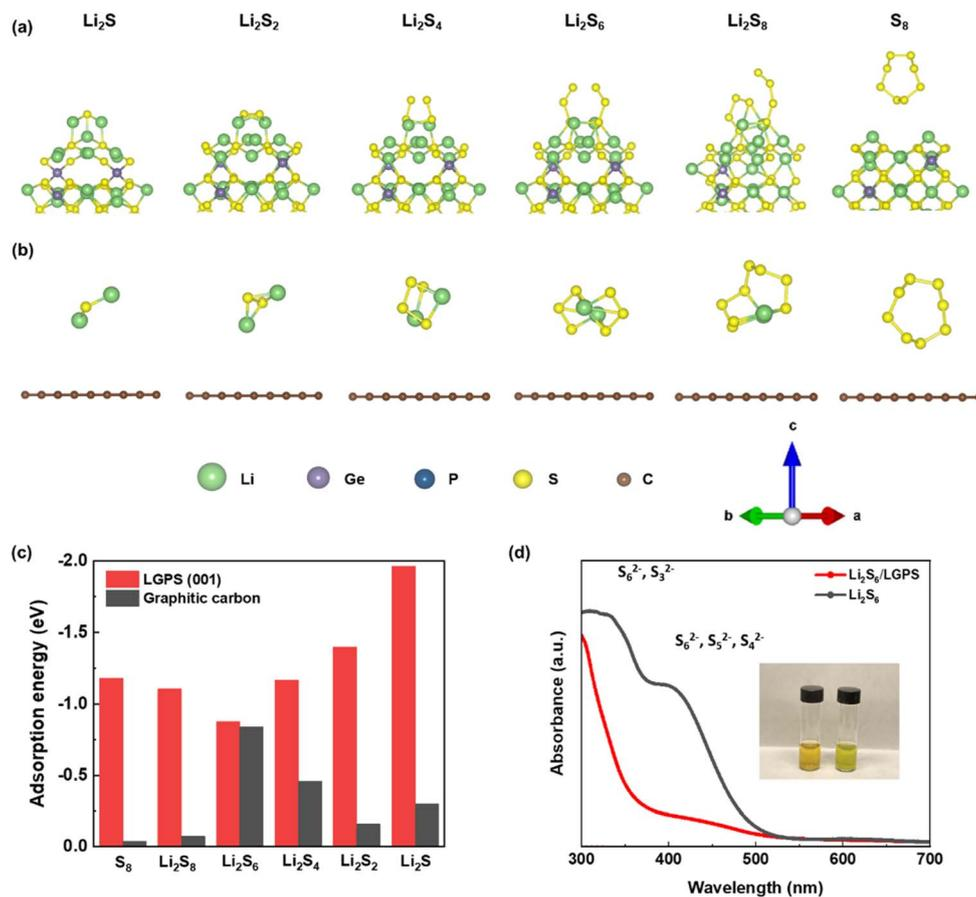
Fig. 2 The adsorption configuration of lithium polysulfides and S<sub>8</sub> on (a) LGPS (001) and (b) graphitic carbon. (c) Adsorption energies of lithium polysulfides on LGPS and graphitic carbon. (d) UV-vis spectra of a 5 mM Li<sub>2</sub>S<sub>6</sub> solution before (black line; left photo inset) and after (red line; right photo inset) immersion of LGPS in the solution.
