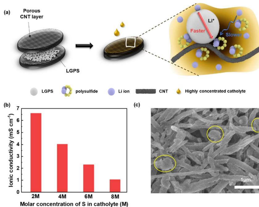
Fig. 1 (a) The cathode was fabricated by sandwiching LGPS particles, followed by the application of a polysulfide solution onto the porous structure. While lithium ions are readily transported through LGPS, their movement is sluggish through the lean polysulfide electrolyte. (b) The ionic conductivity of 2 M, 4 M, 6 M and 8 M catholyte. (c) The scanning electron microscopy (SEM) image of a CNT/LGPS electrode with distributed LGPS particles after cycling.
