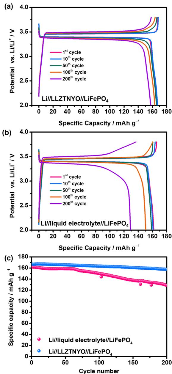
Fig. 10 (a) Galvanostatic charge/discharge curve of (a) Li//LLZTNYO//LiFePO<sub>4</sub> and (b) Li//liquid electrolyte//LiFePO<sub>4</sub> cells in the voltage potential range of 2–3.8 V vs. Li/Li<sup>+</sup>. (c) Cycling performance at 0.1C of Li//LLZTNYO//LiFePO<sub>4</sub> and Li//liquid electrolyte//LiFePO<sub>4</sub> cells.
