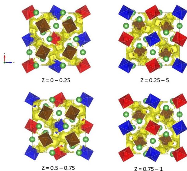
Fig. 2 Bond valence sum (BVS) map of lithium ions for  $\text{Li}_{6.5}\text{La}_3\text{Zr}_{0.5}\text{Ta}_{0.5}\text{Nb}_{0.5}\text{Y}_{0.5}\text{O}_{12}$ . The lithium-ion percolation network was represented by a yellow contour plot. Projections with different  $z$  values were selected to avoid structural overlapping.
