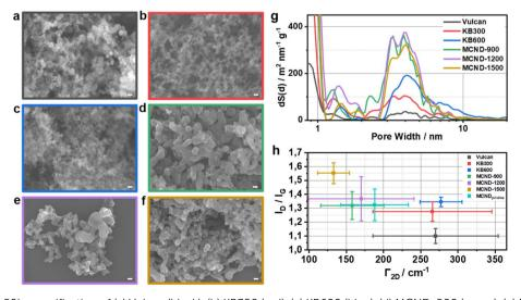
Fig. 1 SEM images at 50k magnification of (a) Vulcan (black), (b) KB300 (red), (c) KB600 (blue), (d) MCND-900 (green), (e) MCND-1200 (purple), and (f) MCND-1500 (gold); the scale bar represents 100 nm; (g) pore size distribution by QSDFT (quenched solid density functional theory) of  $N_2$ physisorption (N2 carbon adsorption branch kernel at 77 K for slit/cylindrical pores); (h) statistical Raman spectroscopy (SRS) spectra of all six samples and pristine MCNDs (unannealed, turquoise).
