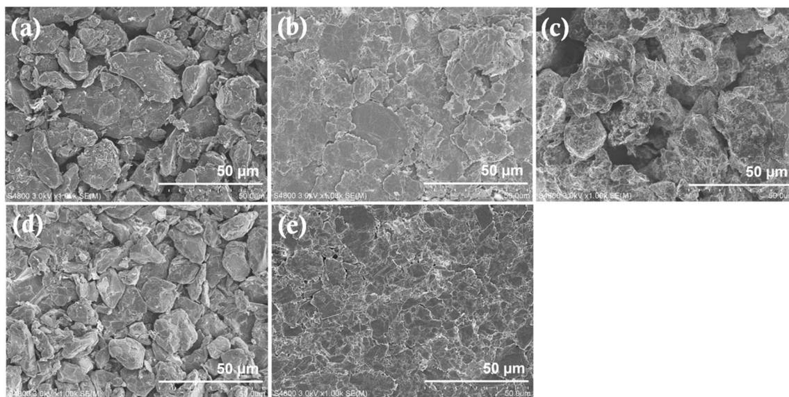
Fig. 3 SEM images of the (a) Gr-W (b) Gr-AcOH (c) Gr-KOH and (d) Gr-N<sub>2</sub> (e) Gr-C samples.
