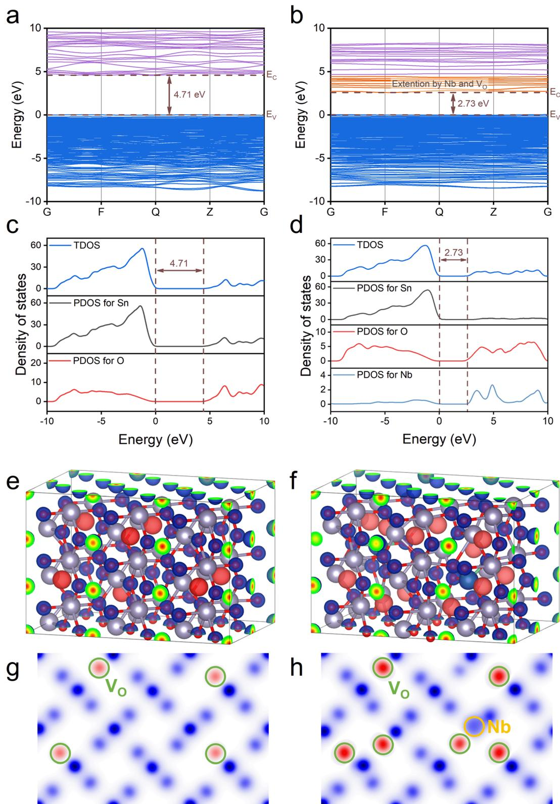
Fig. 4 DFT simulated electrical properties of undoped (left column) and Nb-doped (right column)  $\text{SnO}_2$  super cells with VO: (a and b) band structure; (c and d) TDOS and PDOS; (e and f) differential charge density and (g and h) specific profile with  $\text{V}_\text{O}$  and Nb.
