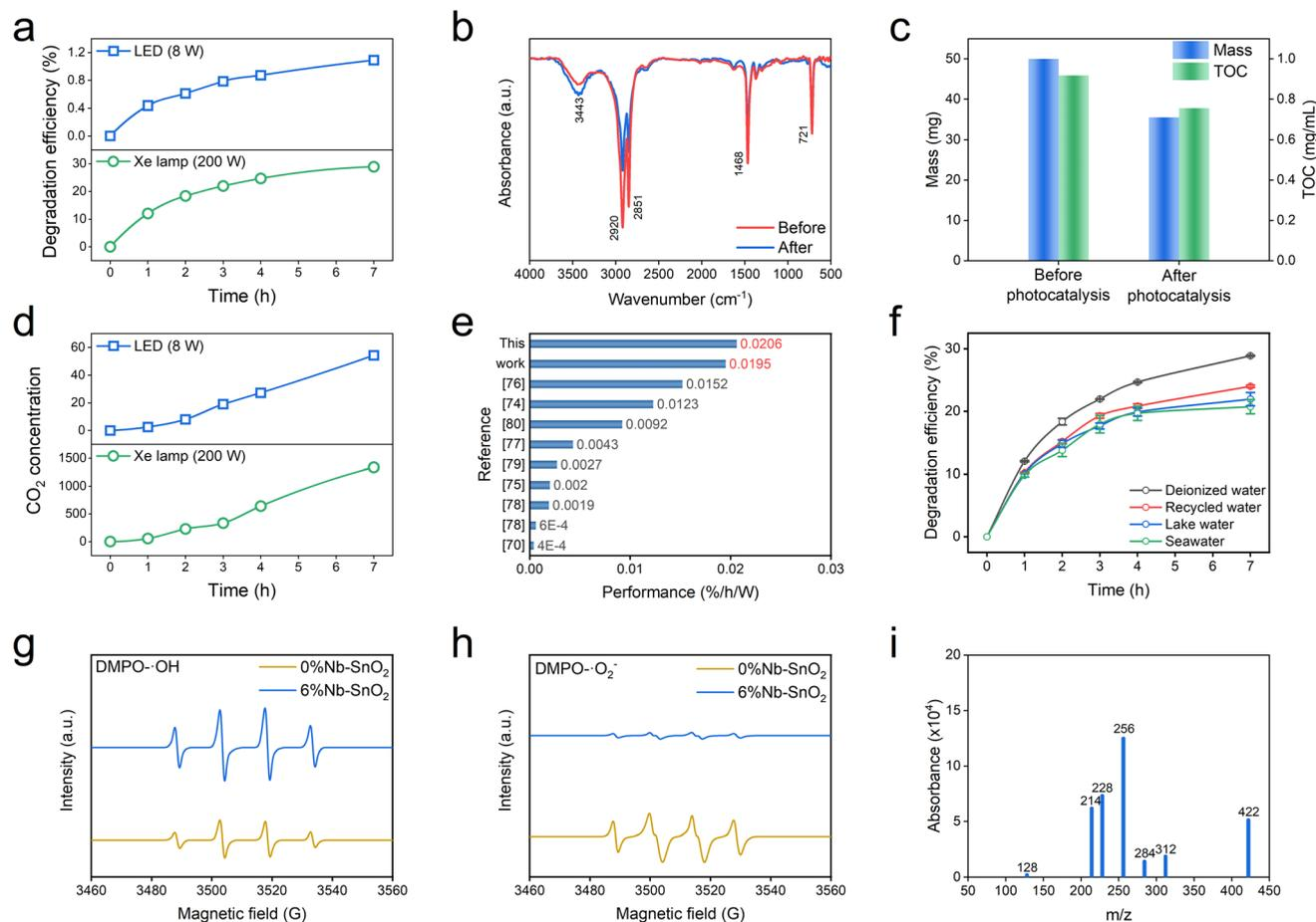
Fig. 5 Photocatalytic degradation of MPs by SnO<sub>2</sub> QDs with Nb-induced VO: (a) degradation efficiency under 8 W and 200 W irradiation; (b) FTIR spectra before and after 4 h irradiation; (c) mass loss and TOC analysis; (d) CO<sub>2</sub> product amount; (e) performance comparison with other reports; (f) degradation in various realistic aqueous environments; (g) ESR spectra of  $\cdot\text{OH}$ ; (h) ESR spectra of  $\cdot\text{O}_2^-$ ; (i) GC-MS for intermediate determination.
