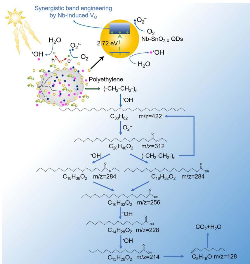
Fig. 6 Pathway and mechanism of visible-light driven photocatalytic degradation of PE by SnO<sub>2</sub> QDs with synergistic band engineering by Nb-induced V<sub>O</sub>.
