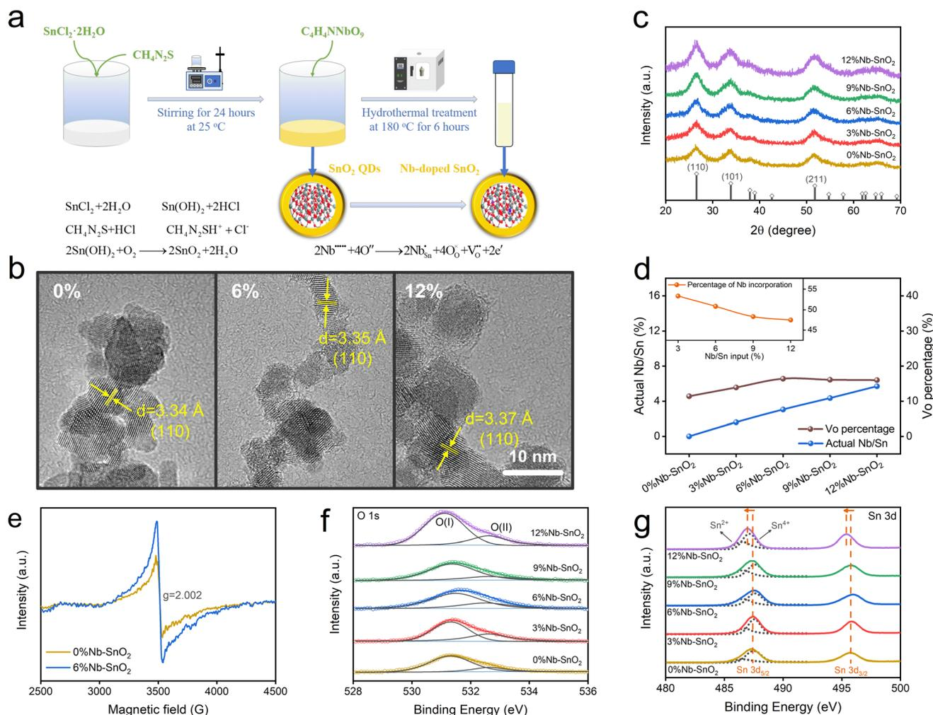
Fig. 1 Synthesis and microstructural properties of SnO<sub>2</sub> QDs with Nb-induced V<sub>O</sub>: (a) schematic illustration of the preparation procedure; (b) HRTEM morphologies; (c) XRD patterns; (d) stoichiometry of SnO<sub>2</sub> QDs with dual defects; (e) ESR spectra; (f) XPS O 1s spectra; (g) XPS Sn 3d spectra.
