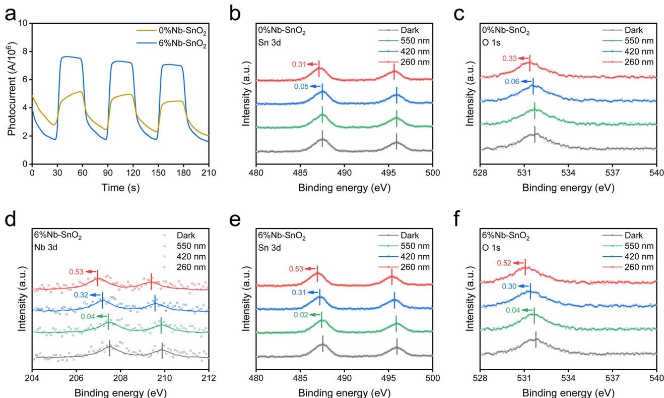
Fig. 3 *In situ* characterization of optical–electrical properties under irradiation: (a) photocurrent; XPS spectra of (b) Sn 3d and (c) O 1s of 0% Nb–SnO<sub>2</sub> and (d) Nb 3d, (e) Sn 3d and (f) O 1s of 6% Nb–SnO<sub>2</sub>.
