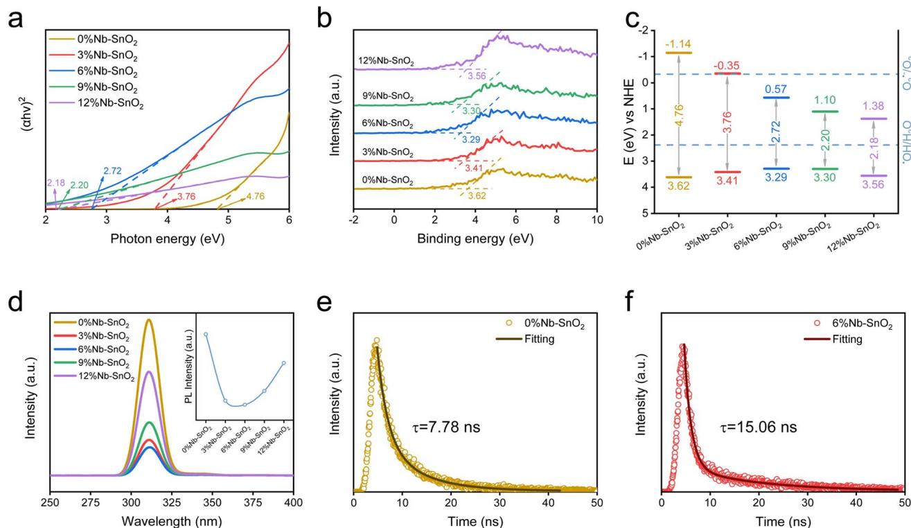
Fig. 2 Band structures and optical–electrical properties of SnO<sub>2</sub> QDs with Nb-induced V<sub>O</sub>: (a) Tauc plots for bandgap evaluation; (b) XPS valence band spectra; (c) band structures; (d) photoluminescence spectra; TRPL spectra for evaluation of the carrier lifetime of (e) 0% Nb–SnO<sub>2</sub> and (f) 6% Nb–SnO<sub>2</sub>.
