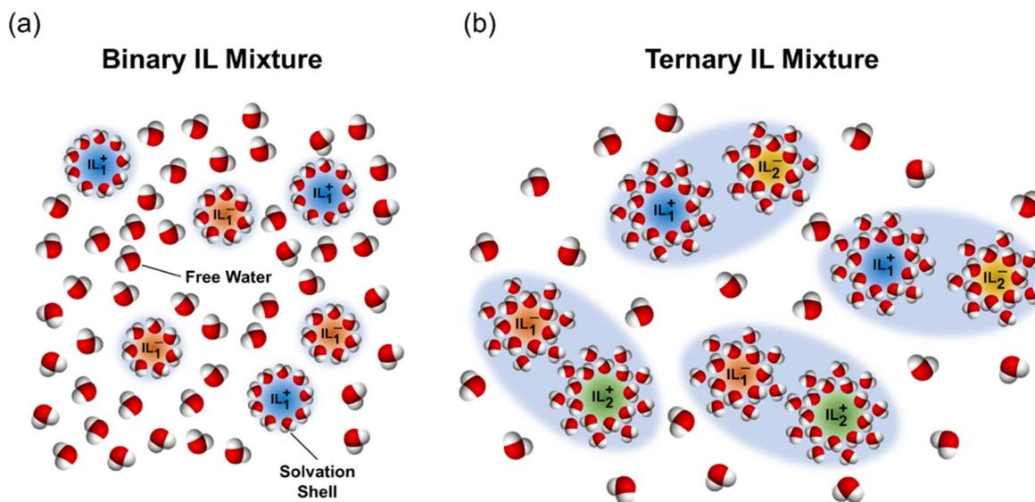
Fig. 8 Illustration of the hypothesized ion association interaction mechanism between two IL species in a ternary mixture that promotes a decrease in  $T_C$  coupled with an increase in osmolality. (a) Binary IL mixtures. (b) Ternary IL mixtures. The decrease in the number of free water molecules through solvation within the ion clusters results in an increase in osmolality, while further decreasing the entropy of mixing due to increased molecular ordering, effectively lowering  $T_C$ .
