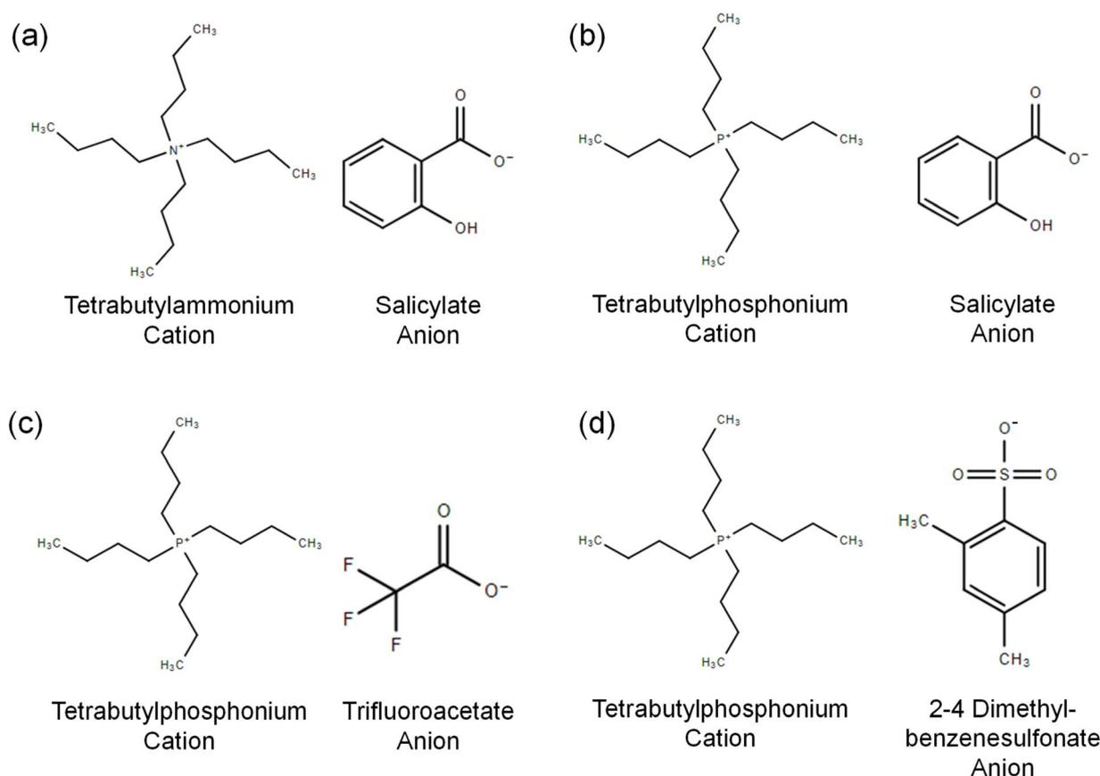
Fig. 3 Chemical structures of the ionic liquids studied in this work and their molar masses ( $M$ ). (a) NSal ( $M_{\text{NSal}} = 364.11 \text{ g mol}^{-1}$ ). (b) PSal ( $M_{\text{PSal}} = 396.54 \text{ g mol}^{-1}$ ). (c) PTFA ( $M_{\text{PTFA}} = 372.02 \text{ g mol}^{-1}$ ). (d) PDMBS ( $M_{\text{PDMBS}} = 458.25 \text{ g mol}^{-1}$ ).
