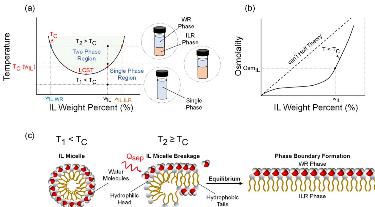
Fig. 1 Overview of LCST behavior. (a) Binodal phase diagram showing LCST behavior in IL–water mixtures. (b) Osmolality as a function of IL concentration in an aqueous solution at a temperature below  $T_C$  (single-phase mixture). (c) Illustration of IL–water micelle formation at temperatures below  $T_C$ , which upon heating causes the micelles to break and expose the hydrophobic tails of the IL, resulting in the formation of a phase boundary and two phases (WR and ILR).
