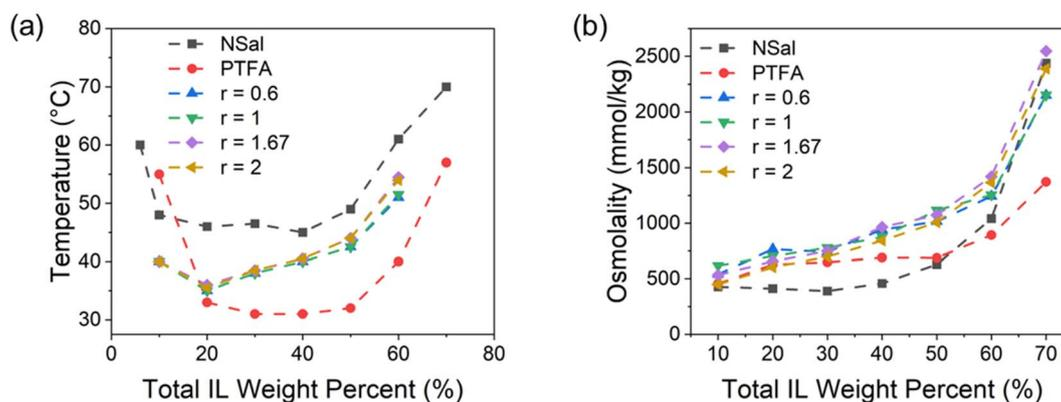
Fig. 7 Properties of NSal + PTFA ternary mixtures as a function of different weight ratios,  $r$ . (a) Phase diagrams of the mixtures as well as pure NSal and PTFA. (b) Osmolality of the ternary mixtures as well as pure NSal and PTFA. All osmolality measurements shown in (b) are based on five water activity measurements with a maximum standard deviation of  $\pm 16\%$  in osmolality. The maximum error in the cloud point measurements for  $T_C$  shown in (a) is 0.5 °C.
