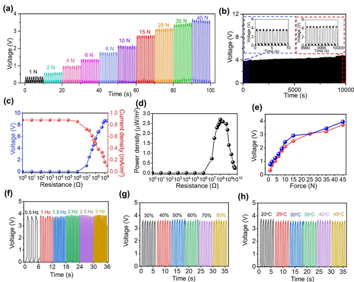
Fig. 3 Electrical characterization of the TENG sensor. (a) Force response. (b) Long-term stability ( $10\,000$  s). (c) Voltage and current density variation with resistance. (d) Power density variation with resistance. (e) Hysteresis curve. (f) TENG output response with frequency variation. (g) Humidity variation effect on TENG output. (h) Temperature variation effect on TENG output.
