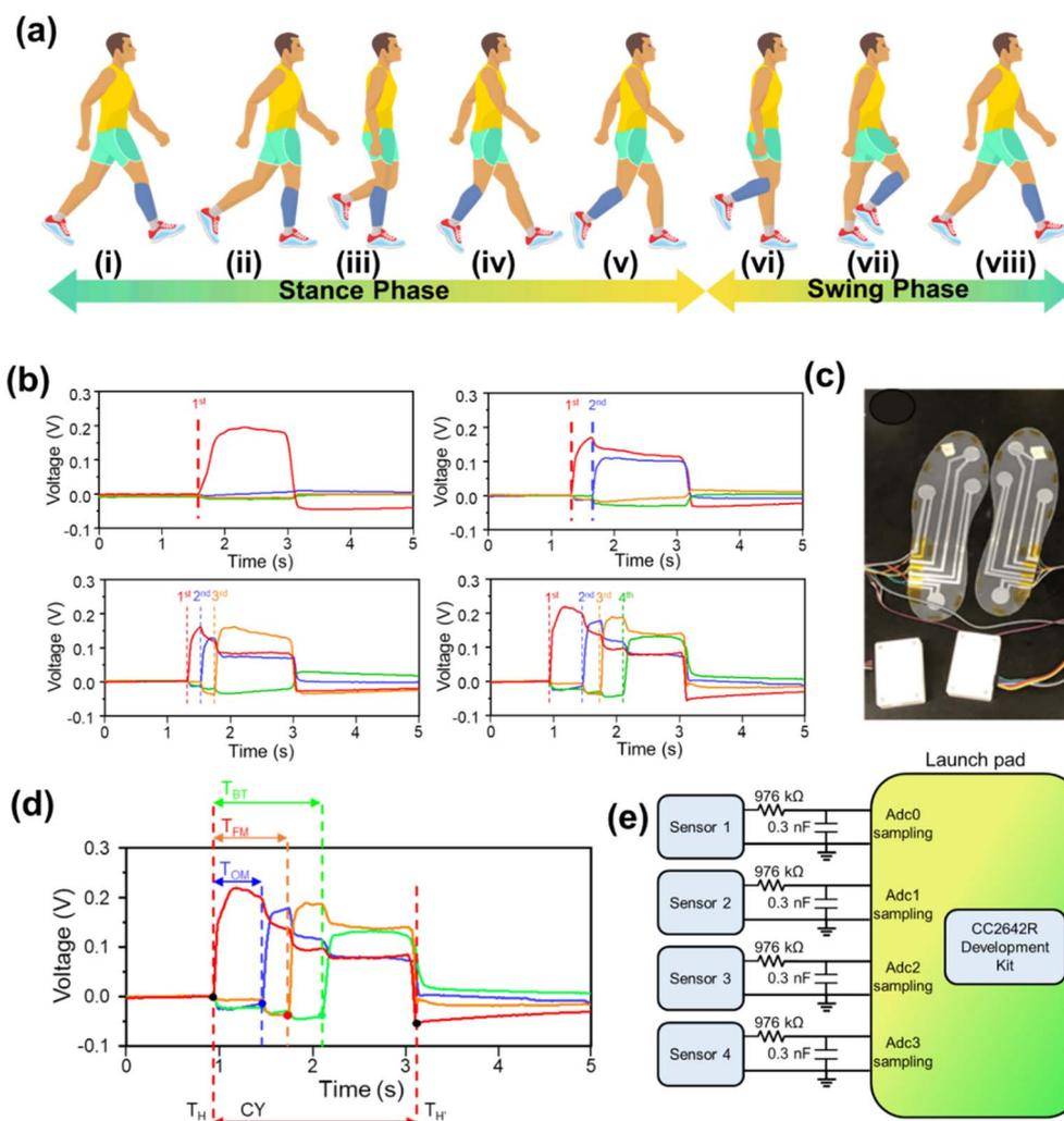
Fig. 4 Human gait cycle and real-time sensor data acquisition. (a) Typical human gait cycle-stance and swing phases. (b) Dynamic response profiles of the four TENG sensors (1<sup>st</sup>, 2<sup>nd</sup>, 3<sup>rd</sup>, and 4<sup>th</sup>) under actuation. (c) Image of the insoles with TENG sensors and DAQ. (d) Time-domain diagnostic model depiction. (e) Illustration of the CC2652R1FRGZ MCU-based DAQ system.
