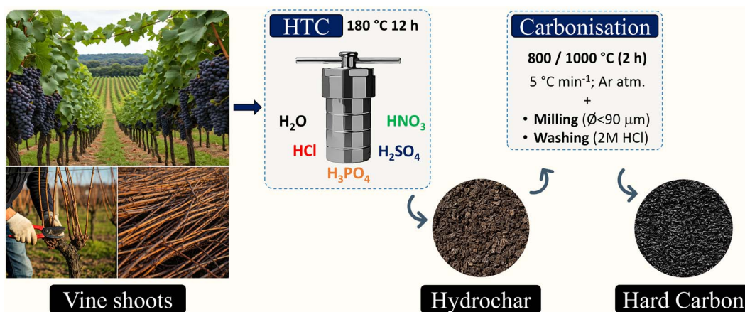
Fig. 1 Graphical summary of the hard carbon synthesis via HTC.
