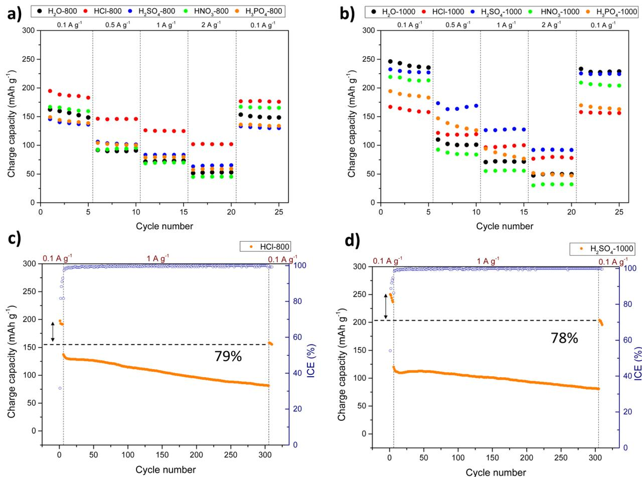
Fig. 5 (a and b) Specific charge capacities vs. cycle number at various current densities ranging from 0.1 to 2 A g<sup>-1</sup> and (c and d) cycling performance of HCl-800 and H<sub>2</sub>SO<sub>4</sub>-1000 for 300 cycles at 1 A g<sup>-1</sup> in NaTFSI/EC:DMC.
