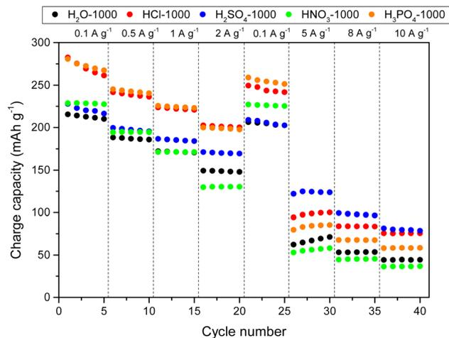
Fig. 6 Specific charge capacities vs. cycle number at various current densities ranging from 0.1 to 10 A g<sup>-1</sup> in NaPF<sub>6</sub>/DGM.
