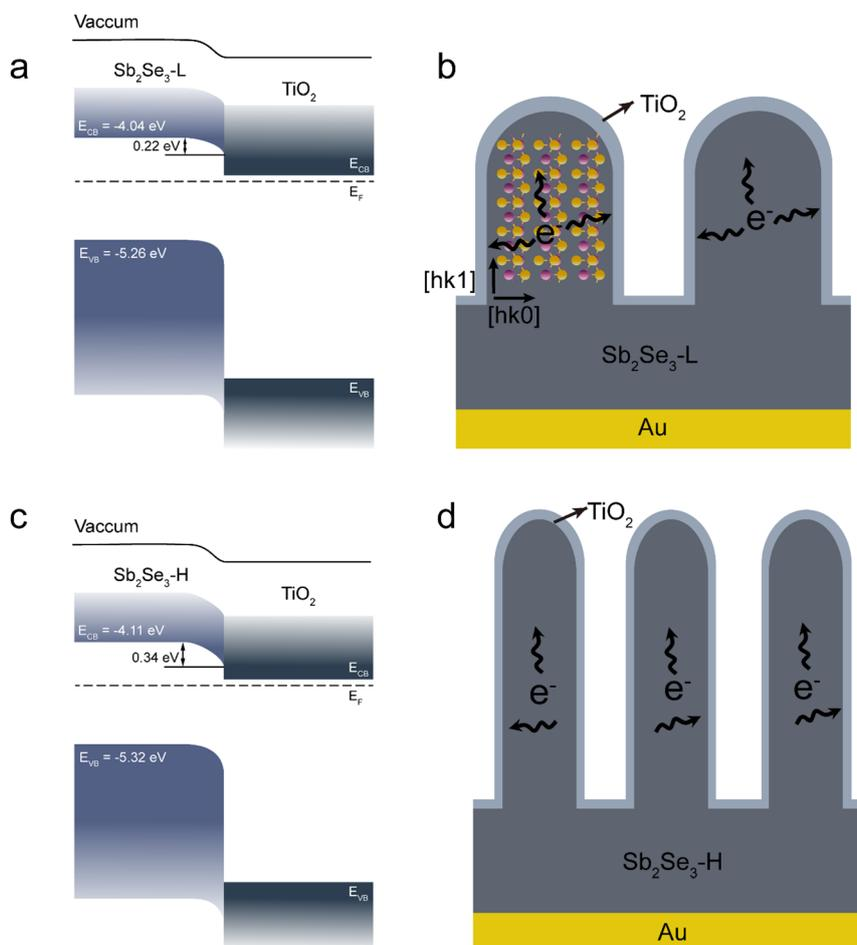
Fig. 5 Band diagram of the (a) Sb<sub>2</sub>Se<sub>3</sub>-L and (c) Sb<sub>2</sub>Se<sub>3</sub>-H photocathodes. Schematic illustration of the charge separation mechanism in the (b) Sb<sub>2</sub>Se<sub>3</sub>-L and (d) Sb<sub>2</sub>Se<sub>3</sub>-H photocathodes.
