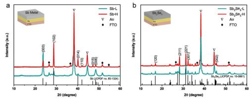
Fig. 1 (a) XRD pattern of Sb metal deposited at substrate temperatures of 25 °C and 75 °C. (b) XRD pattern of Sb<sub>2</sub>Se<sub>3</sub> synthesized at 325 °C for 30 min by selenizing the corresponding Sb metal sample. The configuration of the samples used for XRD measurement is provided in the inset.
