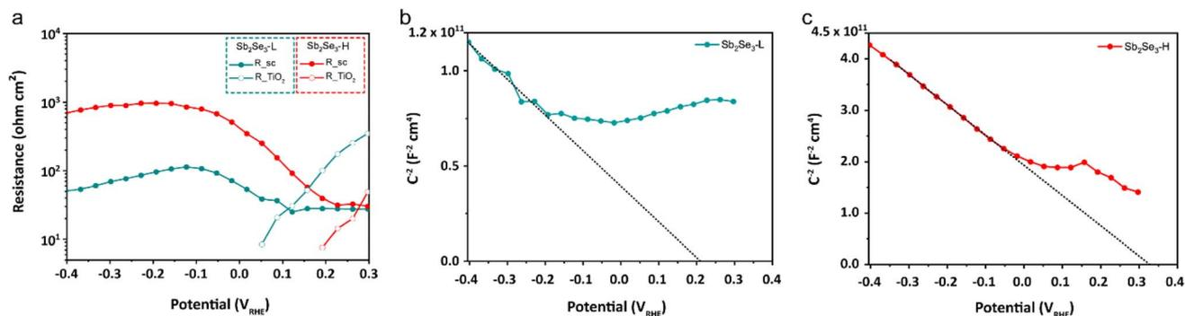
Fig. 4 (a) Resistances of the Sb<sub>2</sub>Se<sub>3</sub>-L and Sb<sub>2</sub>Se<sub>3</sub>-H photocathodes from the EIS fitting procedure under 10% white light illumination. Mott-Schottky plots of the (b) Sb<sub>2</sub>Se<sub>3</sub>-L and (c) Sb<sub>2</sub>Se<sub>3</sub>-H photocathodes obtained from EIS fitting under dark conditions.
