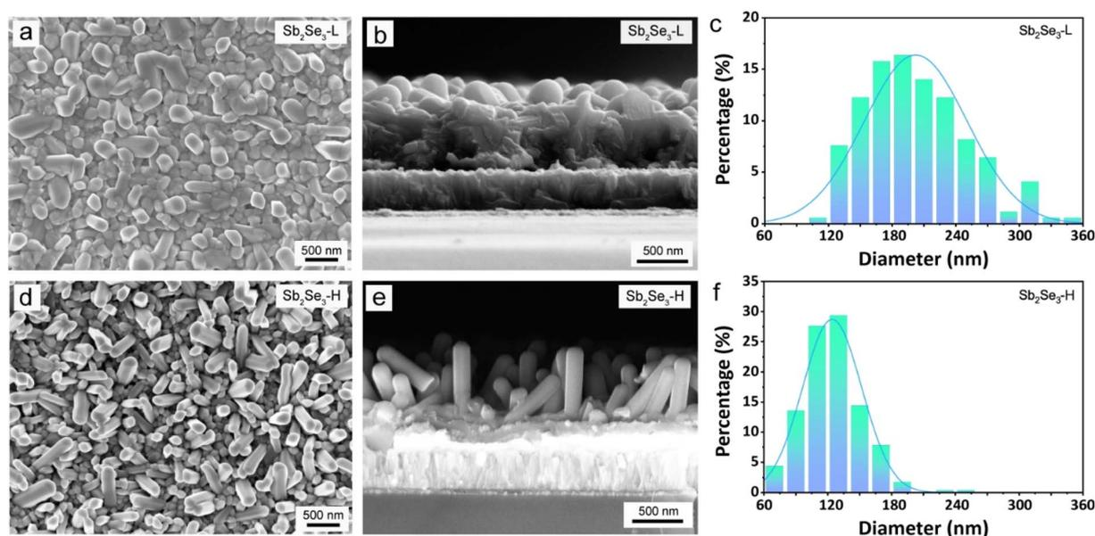
Fig. 2 Top view (a and d) and cross-sectional view (b and e) SEM images of the (a and b)  $\text{Sb}_2\text{Se}_3$ -L and (d and e)  $\text{Sb}_2\text{Se}_3$ -H thin films. Columnar plots of the characteristic nanorod diameters of the (c)  $\text{Sb}_2\text{Se}_3$ -L and (f)  $\text{Sb}_2\text{Se}_3$ -H thin films.
