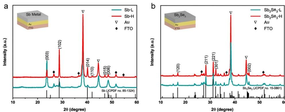
Fig. 1 (a) XRD pattern of Sb metal deposited at substrate temperatures of 25 °C and 75 °C. (b) XRD pattern of  $\text{Sb}_2\text{Se}_3$  synthesized at 325 °C for 30 min by selenizing the corresponding Sb metal sample. The configuration of the samples used for XRD measurement is provided in the inset.
