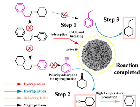
Scheme 2 Proposed reaction pathway for the PPE conversion over the Ni 9 Fe 1 /NiAlO 2 catalyst.
