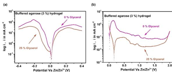
Fig. 5 (a) Stability of Zn metal and (b) carbon coated Ni current collector in the buffered 3% agarose hydrogel electrolyte containing 1 M Zn<sup>2+</sup> without glycerol and in the presence of 25% glycerol (replacing the water in the hydrogel).
