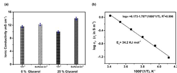
Fig. 4 (a)  $\sigma_i$  of the buffered and unbuffered 3% agarose hydrogel electrolytes containing  $1\text{ M Zn}^{2+}$  in the absence and presence of glycerol and (b) Arrhenius plot showing  $\sigma_i$  as a function of temperature for the buffered 3% agarose hydrogel electrolyte with  $1\text{ M Zn}^{2+}$  containing 25% glycerol.
