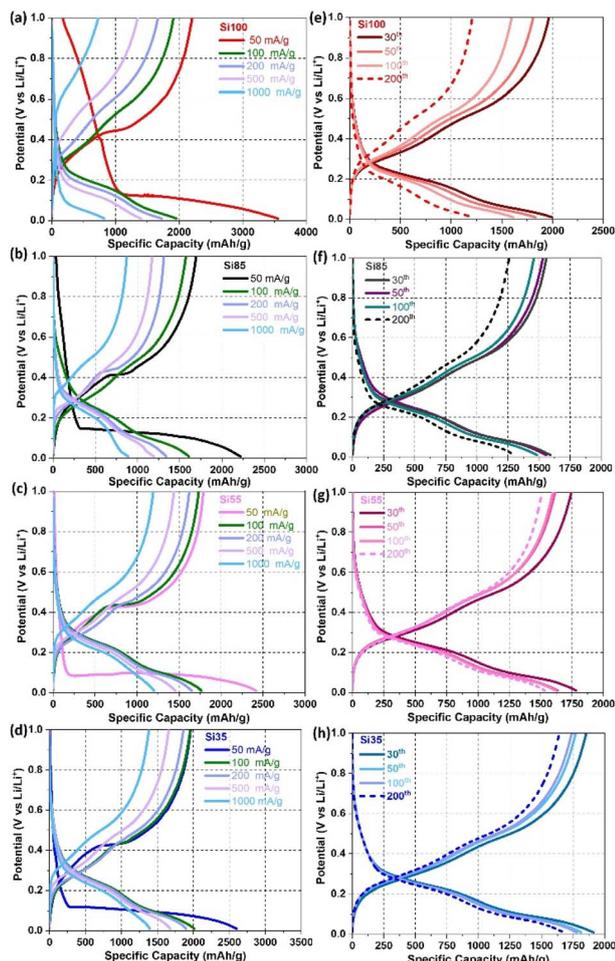
Fig. 4 Voltage–capacity profiles of (a) Si100, (b) Si85, (c) Si55, and (d) Si35 samples when cycled in a range of different applied specific currents from 50 mA g<sup>-1</sup> to 1000 mA g<sup>-1</sup>. A selection of voltage–capacity profiles for long term cycling from the 30<sup>th</sup> to the 200<sup>th</sup> cycle at an applied specific current of 100 mA g<sup>-1</sup> for (e) Si100, (f) Si85, (g) Si55, and (h) Si35 anodes.
