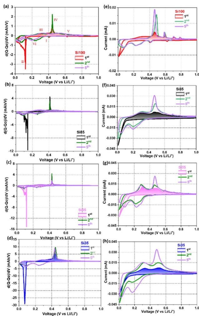
Fig. 5 (a–d) Differential charge curves, and (e–h) CV curves of (red) Si100, (black) Si85, (pink) Si55, and (blue) Si35 at 0.1 mV s<sup>-1</sup> scan rate from 0.01–1.0 V.
