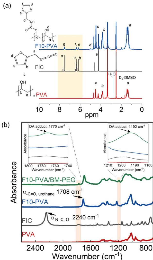
Fig. 1 (a)  $^1\text{H}$  NMR of PVA, FIC, and F10-PVA and (b) ATR-FTIR spectra of PVA, FIC, F10-PVA, and F10-PVA/BM-PEG showing successful attachment of furan groups on PVA and formation of DA bonds. Insets in (b) show the DA adduct peaks at  $1770\text{ cm}^{-1}$  (left) and  $1190\text{ cm}^{-1}$  (right).
