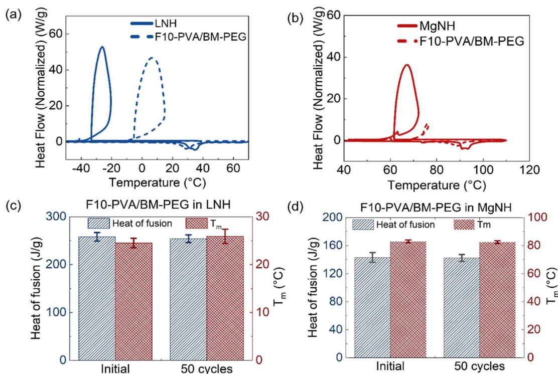
Fig. 7 DSC thermograms showing melting and crystallization transitions in (a) neat LNH and DA salogel, and (b) neat MgNH and DA salogels. Comparison of heat of fusion and melting temperature ( $T_m$ ) in the DA salogel in (c) LNH and (d) MgNH before and after thermal cycling. These experiments were performed with a few grams of DA salogel sealed in a glass vial.
