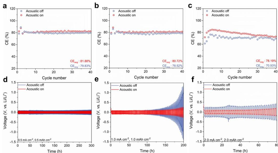
Fig. 3 Comparison of coulombic efficiency for lithium plating/stripping on copper foil at stripping current densities of 0.5 (a), 1.0 (b), and 2.0 mA cm<sup>-2</sup> (c). Voltage-time profiles of Li|Li symmetrical coin cells operated with and without the application of a parallel acoustic field at current densities of 0.5 (d), 1.0 (e), and 2.0 mA cm<sup>-2</sup> (f).
