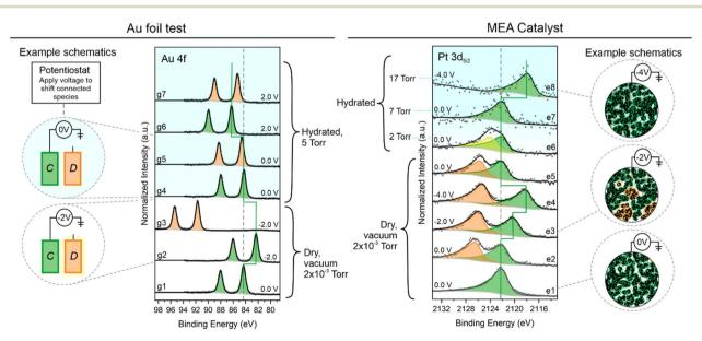
Fig. 4 Particle connectivity trial as a function of potential and condition. Left: Au 4f spectra for an electrically connected (C) and disconnected (D) Au foil. Right: Pt 3d<sub>5/2</sub> XPS results for trials on a Pt-based MEA. Example schematics of the electrical setup are to the side of the spectral regions for some conditions
