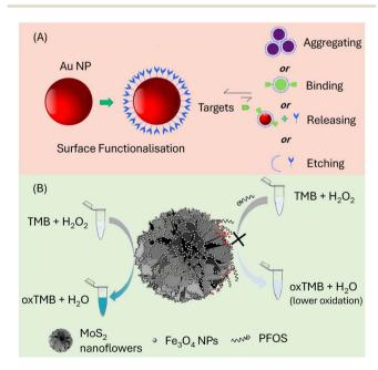
Fig. 5 (A) Illustration of the possible interactions between Au NPs and the target analyte. Reproduced from ref. 64 Copyright 2017, Elsevier. (B) MoS<sub>2</sub>/Fe<sub>3</sub>O<sub>4</sub> nano-flowers for the colorimetric determination of PFAS producing a blue hue when 3,3,5,5-tetramethylbenzidine (TMB) is oxidized in H<sub>2</sub>O<sub>2</sub>. Reproduced from ref. 65 Copyright 2019, Elsevier.
