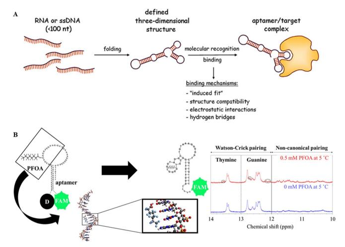
Fig. 14 (A) Schematic of the structure and mechanisms of aptamer target complex formation. Reproduced from ref. 128 Copyright 2013, Swiss Med Wkly. (B) PFOA\_JYP\_2 predicted 2D structures with 0 mM PFOA &ppartial 6 0.5 mM PFOA and 1D- $^1$ H NMR spectra showing the changes in Watson—Crick pairing and non-canonical pairing before and after adding &ppartial 6 0.5 mM PFO. Reproduced from ref. 129 Copyright 2022, Elsevier.
