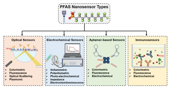
Types of PFAS nano-sensors based on the underlying processes with materials and output signals
