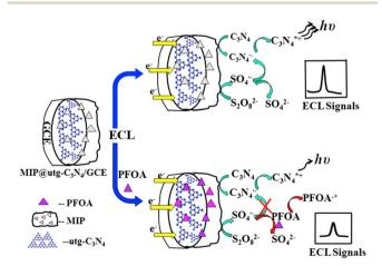
Fig. 13 Illustrative electrochemiluminescence detection technique for PFOA with MIP-functionalized utg-C<sub>3</sub>N<sub>4</sub> in S<sub>2</sub>O<sub>8</sub><sup>2</sup> Reproduced from ref. 105 Copyright 2015, Elsevier.
