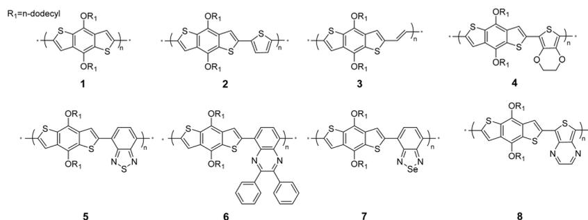
**Fig. 4** Conjugated copolymers **1–8** based on BDT and varied acceptor units.
