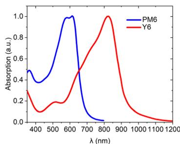
Fig. 11 Complementary absorption of NFA Y6 and PM6 films showing a complementarity of absorption of wide band-gap polymers with NFAs.
