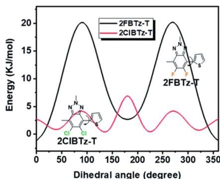
Fig. 15 The twisting barriers of chlorine/fluorine substituted BTz with an adjacent thiophene linker calculated by the DFT method. Copyright 2019 (RSC).<sup>166</sup>
