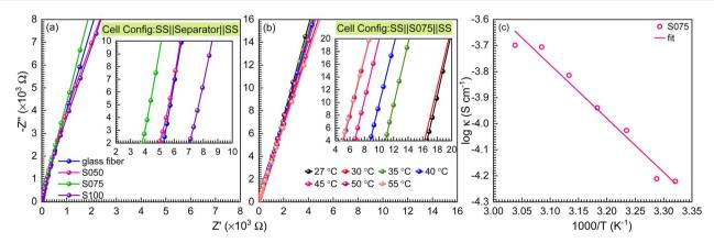
Fig. 4 (a) The Nyquist plot for all the separators at room temperature; (b) the Nyquist plot for the control, S075 membrane at the various temperatures (27 °C, 30 °C, 35 °C, 40 °C, 50 °C, 50 °C, 55 °C), using a blocking electrode system (SS||separator||SS); (c) the ionic conductivity values for the S075 separator at the different temperatures.
