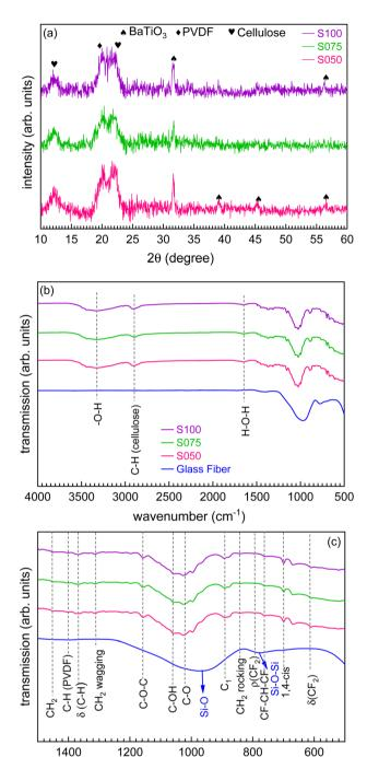
Fig. 1 (a) The X-ray diffraction patterns of the S050, S075 and S100 paper separators, and (b) the ATR-FTIR spectra for all the separators (glass fiber, S050, S075 and S100). (c) The zoomed view between 500 and 1500 cm<sup>-1</sup>.
