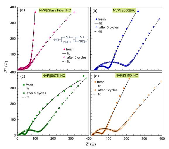
Fig. 6 (a-d) The Nyquist plots for the NVP-HC full cells with glass fiber, and paper separators (\$050, \$075 and \$100) for the fresh and after stabilizing the SEI at 0.1C for five cycles, along with the fitting using the Randles circuit shown in the insets.
